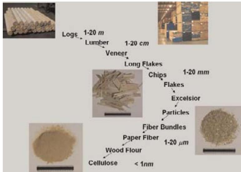
Fig. 14. Basic wood elements, from largest to smallest.
