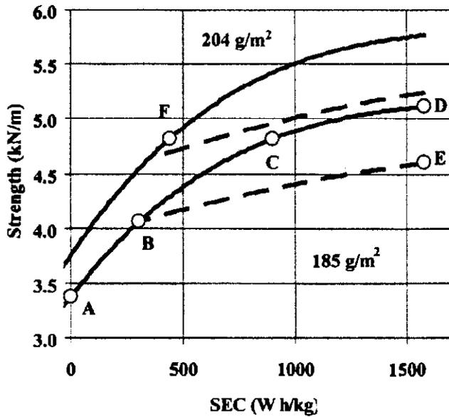
Figure 7. Variation of microplate strength with SEC of refining and dependence on flute size for linerboard at two BW levels. Lower plot (points A–E), 185-g/m<sup>2</sup> linerboard; upper plot (point F), 204-g/m<sup>2</sup> linerboard. Solid lines, predicted  $P_u$  in B- or C-flute corrugated structure; dashed lines, predicted  $B_u$  in A-flute structure.
