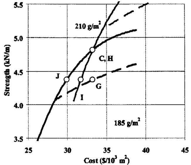
Figure 9. Variation of microplate strength with combined cost components of fiber at  $C_F = \$140/t$  and energy at  $C_E = 5$  cents/kW·h and dependence on flute size for linerboard at two BW levels. Lower plot (points C, J, G), 185-g/m<sup>2</sup> linerboard; upper plot (points H, I), 210-g/m<sup>2</sup> linerboard. See Figure 7 for explanation of line patterns.
