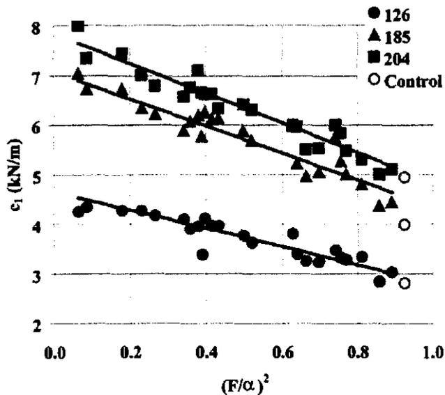
**Figure 2.** Variation of compressive load-strain constant  $c_1$  with freeness ratio  $F/\alpha$  among data in Table 1. Points represent respective mechanical property determined from handsheet at actual basis weight (BW). Lines are predicted property via Eq. (5) based on nominal BW. Legend refers to nominal BW ( $g/m^2$ ) and control material (Table 1).
