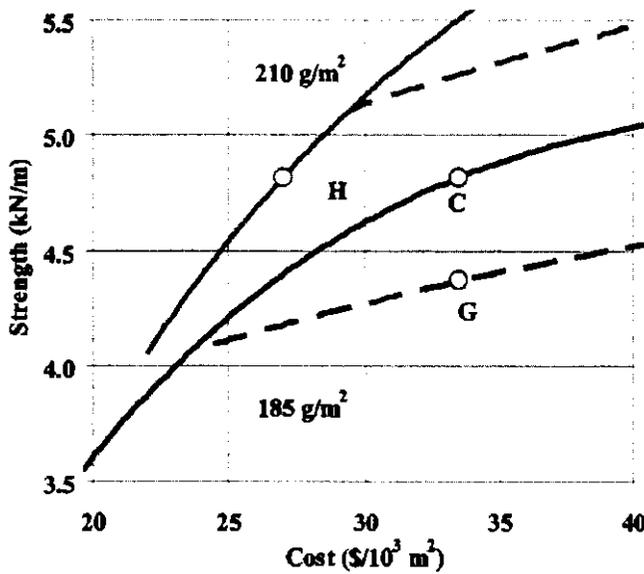
Figure 8. Variation of microplate strength with combined cost components of fiber at  $C_F = \$100/t$  and energy at  $C_E = 9$  cents/kW·h and dependence on flute size for linerboard at two BW levels. Lower plots (points C, G), 185-g/m<sup>2</sup> linerboard; upper plot (point H), 210-g/m<sup>2</sup> linerboard. See Figure 7 for explanation of the line patterns.
