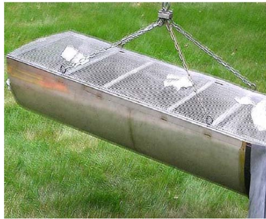
Figure 1 - Unit containing bark-based filtration sorbent in each compartment
