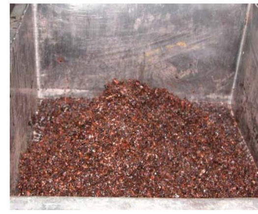
Figure 4 - Alum-infused bark before air-drying
