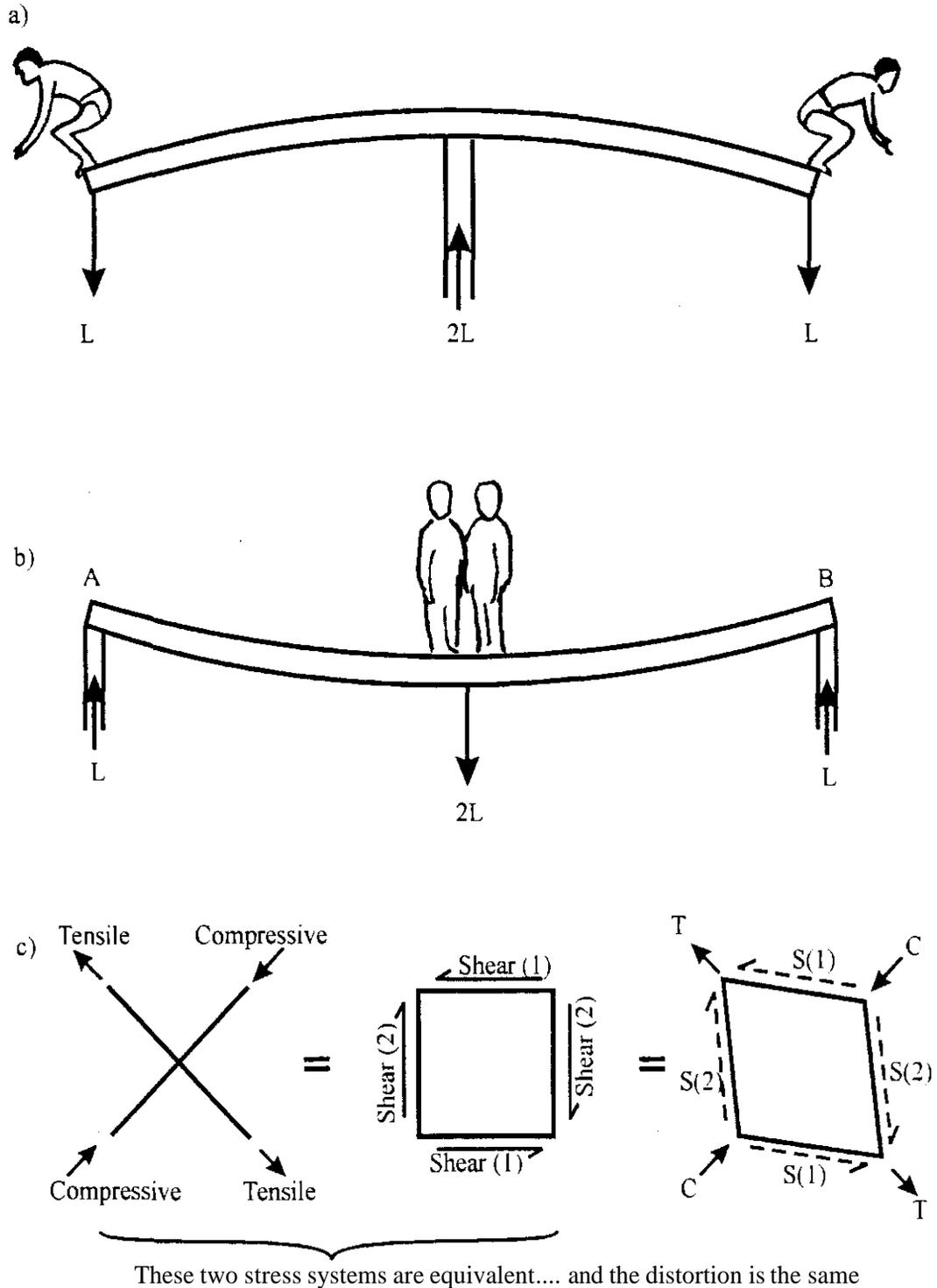
Figure 10.5. A beam under load is equivalent to two cantilevers placed back-to-back and rotated through  $180^\circ$ . Diagonal tensile and compressive stresses in a cantilevered girder are identical to two shear forces acting horizontally and vertically within a solid cantilever or beam. The effect of both stress systems is the same, deforming a square of material into a diamond (Gordon, 1973).
