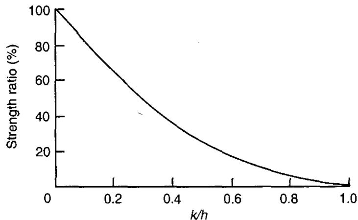
Figure 10.12. Relationship between bending strength ratio and the size of an edge knot expressed as fraction of the face width:  $k$  is knot size;  $h$ , the width of face containing the hot.
