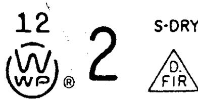
Figure 10.13. An example of a grade stamp for visually graded No. 2 Douglas fir, surfaced dry and produced by mill #12 of the Western Wood Products Association. Reproduced with permission.
