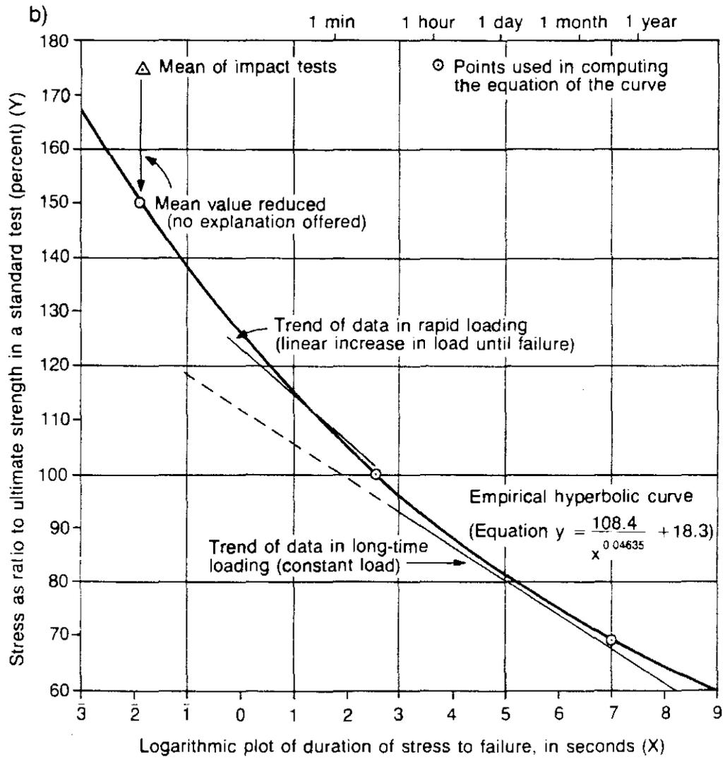
an immediate elastic recovery, a smaller delayed elastic recovery and an irrecoverable component. This time-dependent phenomenon is known as creep. Creep under a long-term constant load results in a long-term deflection that is roughly twice the initially observed elastic deflection. With higher stress levels, above about 55% of the short-term ultimate stress, the creep rate declines gradually before passing through a point of inflection and accelerating again (Figure 10.17a).
