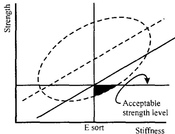
*Figure 10.16.* Schematic E sort. (a) A regression line used as the predictor for four categories: (1) accepted correctly; (2) accepted incorrectly; (3) rejected correctly; and (4) rejected correctly. (b) With the lower confidence line used as the predictor, then a relatively low proportion of material lies in the 'accepted incorrectly' category (lower right).
