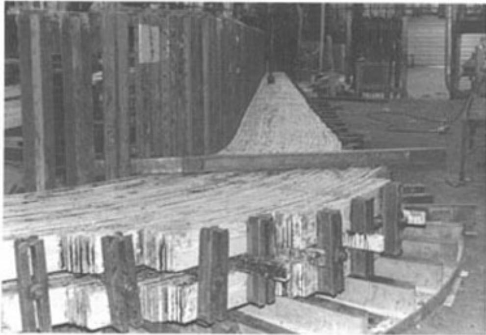
*Figure 10.21.* After being assembled in the clamping bed, the laminations of this Tudor arch are forced together and into shape with a manual air-driven screw clamp.
