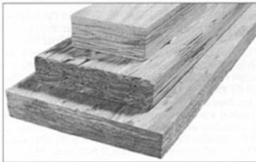
*Figure 10.18.* Three examples of structural composite lumber (top to bottom): laminated veneer lumber (LVL), parallel strand lumber (PSL), and oriented strand lumber (OSL).
