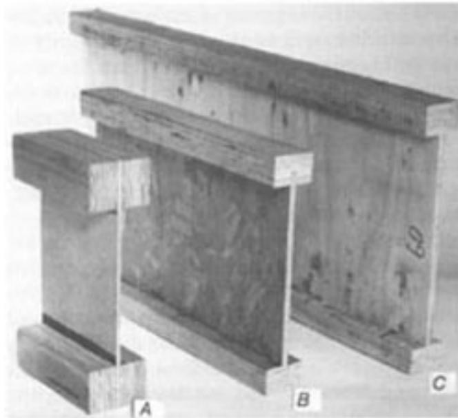
*Figure 10.10.* Prefabricated I-joists with laminated veneer lumber flanges and structural panel webs. (a) With an experimental hardboard web. (b) With commercially produced oriented strandboard web. (c) With a plywood web.
