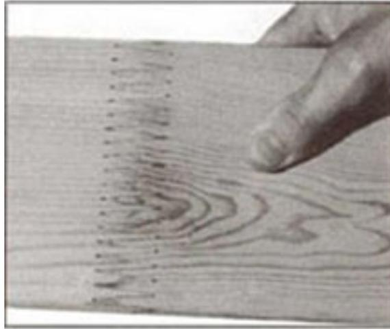
*Figure 10.20.* Typical fingerjoint used in glulam manufacture. The pin-holes at the tips of the fingers are typical of a structural fingerjoint.
