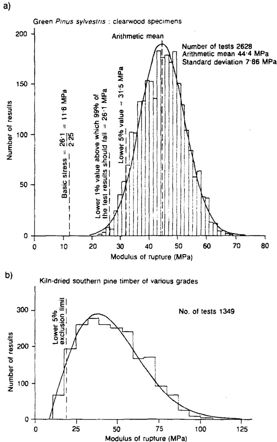
Figure 10.7. Bending strength of clearwood and timber. (a) Small clear green specimens of *Pinus sylvestris* (Sunley, 1968). Data approximates to a normal distribution with a coefficient of variation of 17.7%. Thus 1% of population fails before the stress reaches 26.1 MPa ( $44.4 - 2.33 \times 7.86$ ) and 5% fails below 31.5 MPa ( $44.4 - 1.645 \times 7.86$ ). (b) Variability in bending strength of kiln-dried southern pine of various grades (Doyle and Markwardt, 1966).
