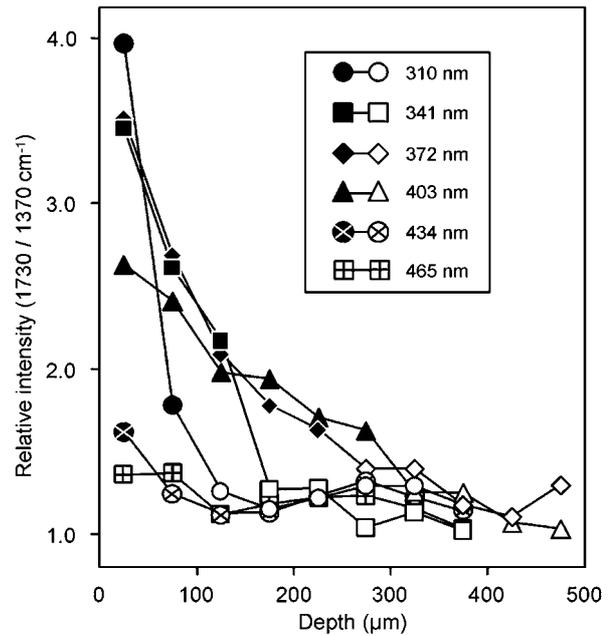
**Figure 4** Changes in absorption at  $1730\text{ cm}^{-1}$  as a function of depth for sugi earlywood exposed to light of different wavelengths from 310 to 465 nm. Filled symbols indicate that significant changes in peaks occurred as a result of exposure of wood to light (difference between unexposed controls and exposed specimens assessed by Smirnov-Grubbs test at the 5% significance level).
