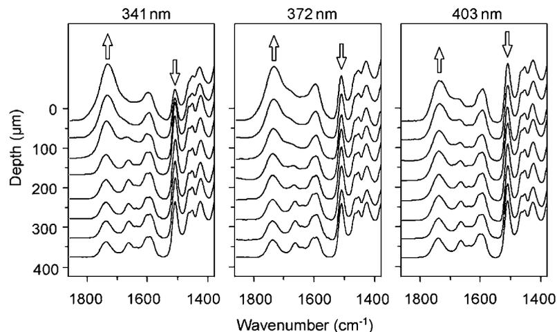
**Figure 3** FT-IR depth profile spectra in the range  $1800\text{--}1400\text{ cm}^{-1}$  of sugi earlywood irradiated with UV radiation at 341 nm (left), 372 nm (middle) or violet light (403 nm, right). Spectra are shown in absorbance units. Arrows indicate where pronounced changes in peak heights occurred.
