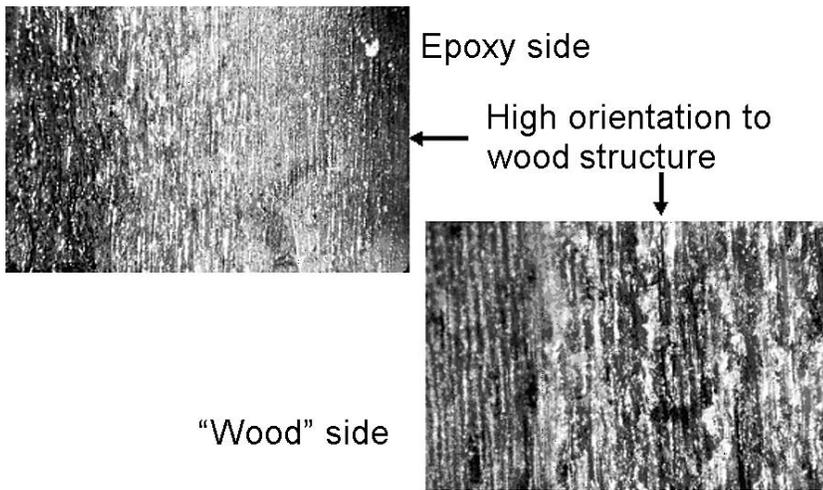
**Figure 1.** ~ Optical microscopy of the failure surface from D 905 testing of a commercial epoxy on wood to illustrate the high orientation on the side mainly covered in epoxy and the side that appears to be bare wood but is not.
