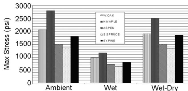
**Figure 4.** ~ Strength determined using ASTM D 905 testing for different wood species and tested for ambient, vacuum pressure soak (wet), and vacuum pressure soak followed by ambient drying (wet-dry) samples. Gradual redrying of D 905 specimen allows recovery of strength.
