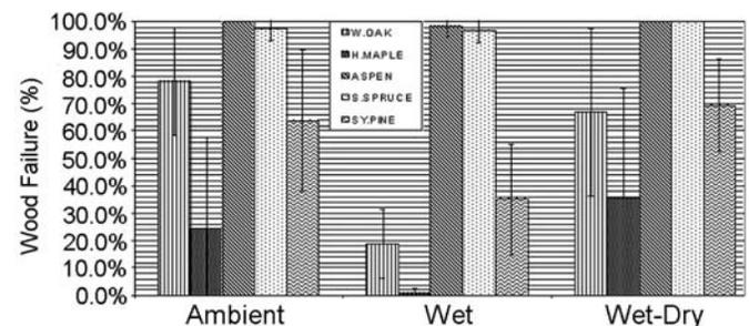
**Figure 5.** ~ Percentage wood failure as determined using ASTM D 905 and ASTM D 5266 testing for different wood species and tested for ambient, vacuum pressure soak (wet), and vacuum pressure soak followed by ambient drying (wet-dry) samples.
