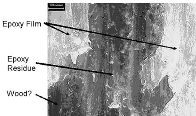
**Figure 2.** ~ Use of fluorescent microscopy showing a specimen similar to that in Figure 1, where the fluorescent epoxy shows up as the lighter color and the non-fluorescent (dark) areas are mainly wood.
