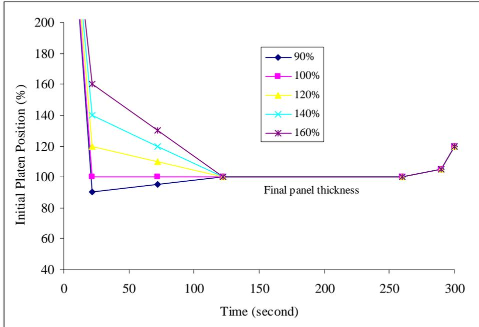
Figure 1. Pressing schedules showing platen position as percentage of final panel thickness over time.
