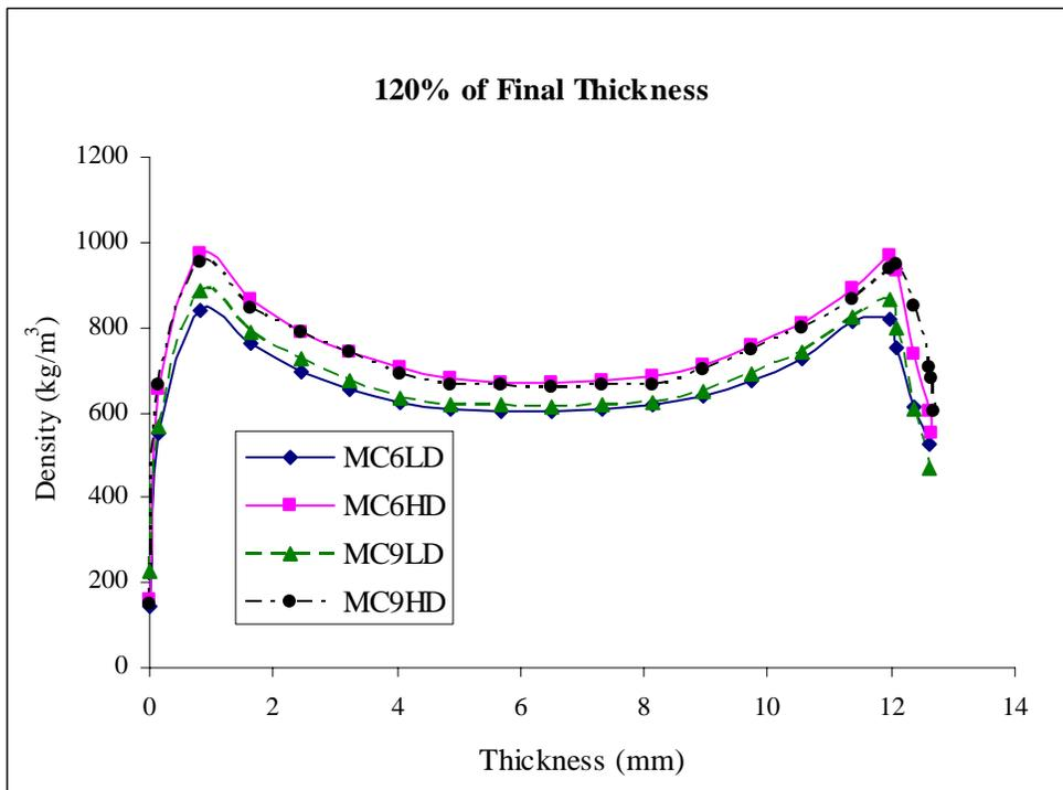
Figure 4. Density profiles with initial platen position at 120% (see Fig. 2 for legend definitions).
