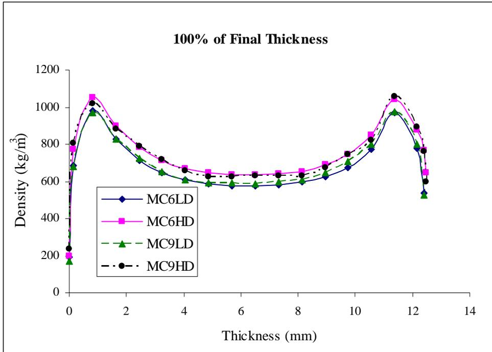
Figure 3. Density profiles with initial platen position at 100% (see Fig. 2 for legend definitions).
