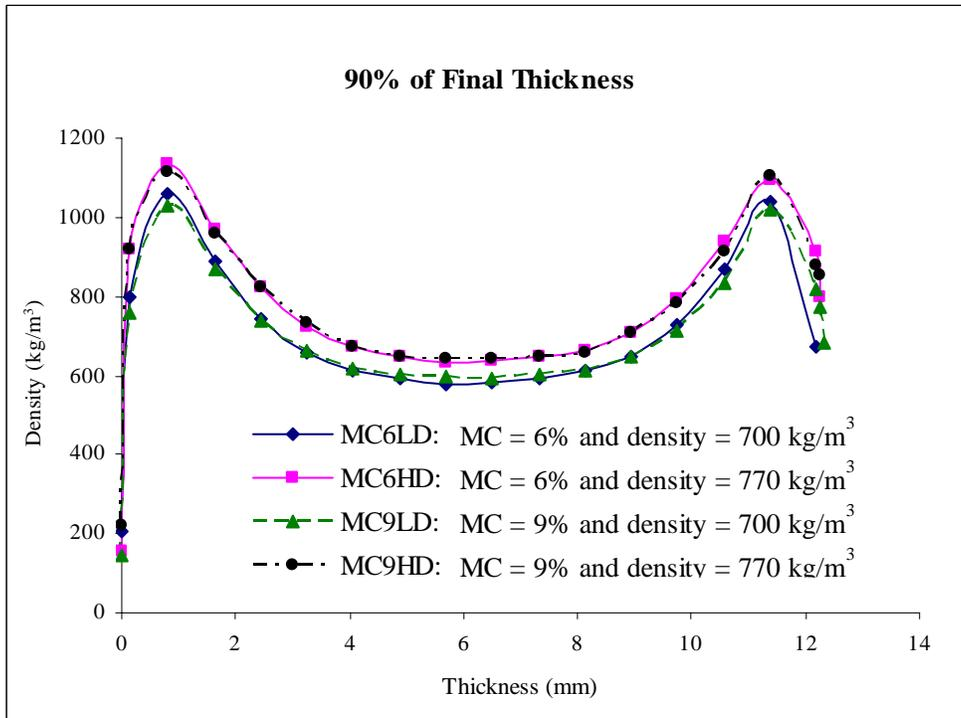
Figure 2. Density profiles with initial platen position at 90% of panel thickness.
