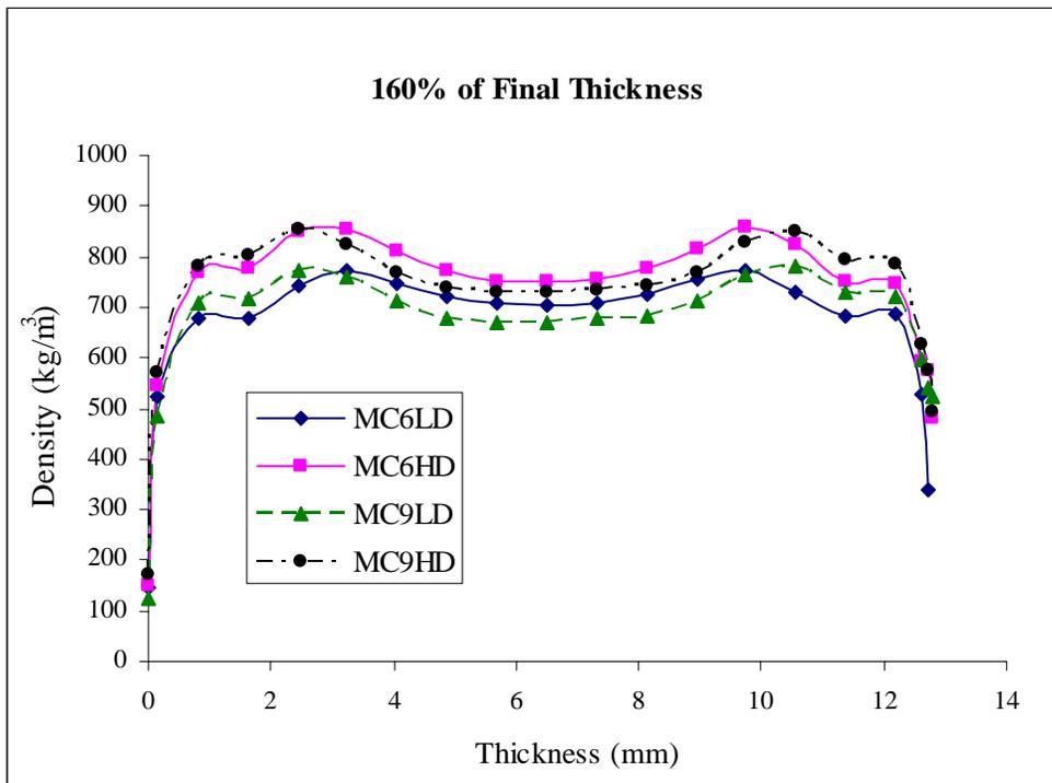
Figure 6. Density profiles with initial platen position at 160% (see Fig. 2 for legend definitions).
