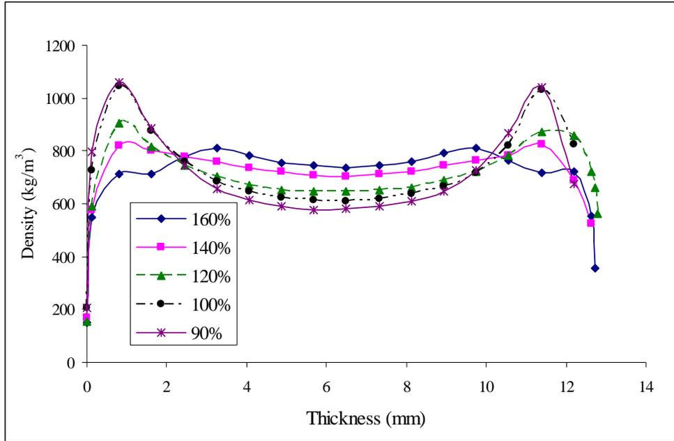
Figure 7. Density profiles with different initial platen positions (see Fig. 2 for legend definitions).
