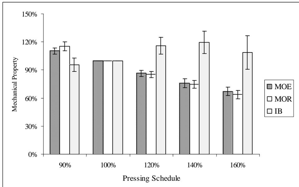
Figure 8. Mechanical properties with different pressing schedules.
