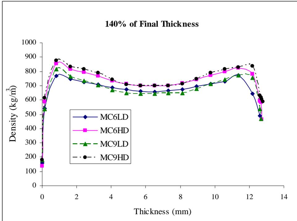
Figure 5. Density profiles with initial platen position at 140% (see Fig. 2 for legend definitions).
