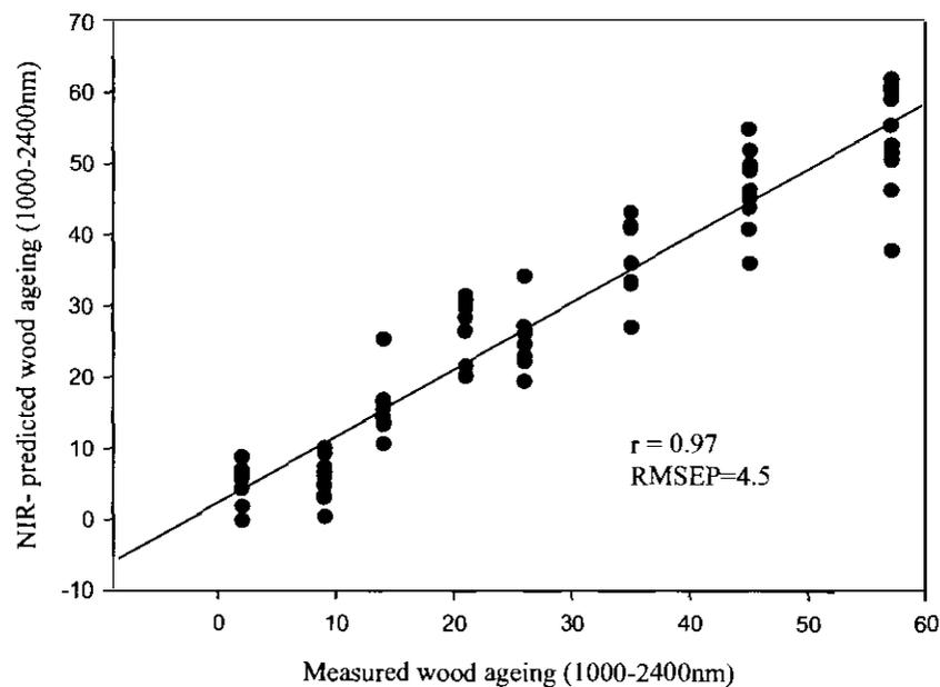
**Figure 4.** Relationship between the actual exposure time and the NIR-predicted exposure time.
