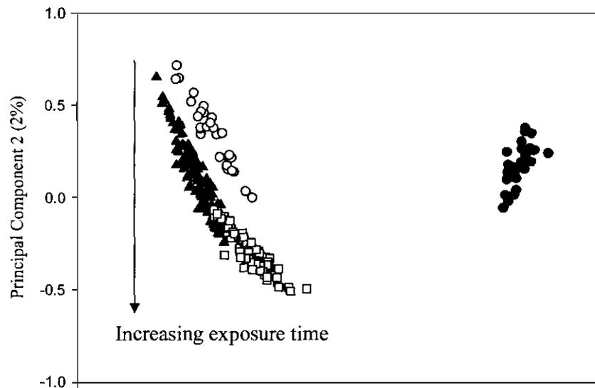
**Figure 3.** Principal component results from NIR spectra collected from the surface of Southern Yellow Pine boards submitted to natural weathering (the symbols correspond to the different exposure time: 0 months – control (●), 2 months (○), 9-14-21-26 months (▲), 35-45-57 months (□))
