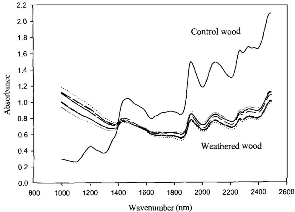
**Figure 1.** Effect of exposure time on infrared spectrum. Exposure months: 2 (long dash), 9 (dotted), 14 (dash-dot-dot), 21 (short dash), 26 (dash-dot), 35 (medium dash), 45 (solid), 57 (gray).
