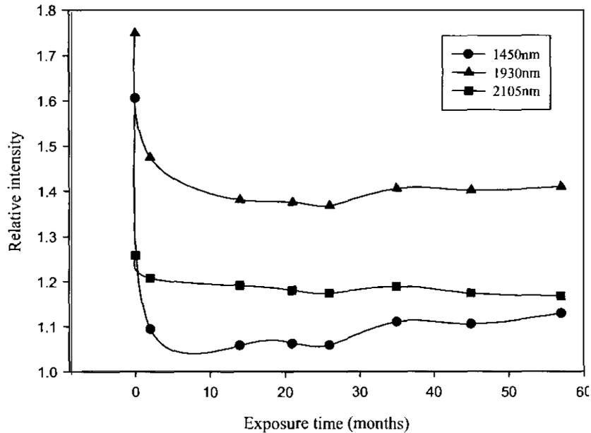
**Figure 2.** Changes of relative absorbance intensity of important chemical groups during weathering of Southern Yellow Pine wood.
