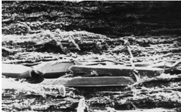
FIGURE 11.23 Scanning electron micrograph of calcium carbonate crystals in lumens of southern pine ( \times 800 ).
