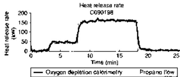
**Fig. 3.** Example of a calibration run for the intermediate scale biomass calorimeter at the University of California Forest Products Laboratory.
