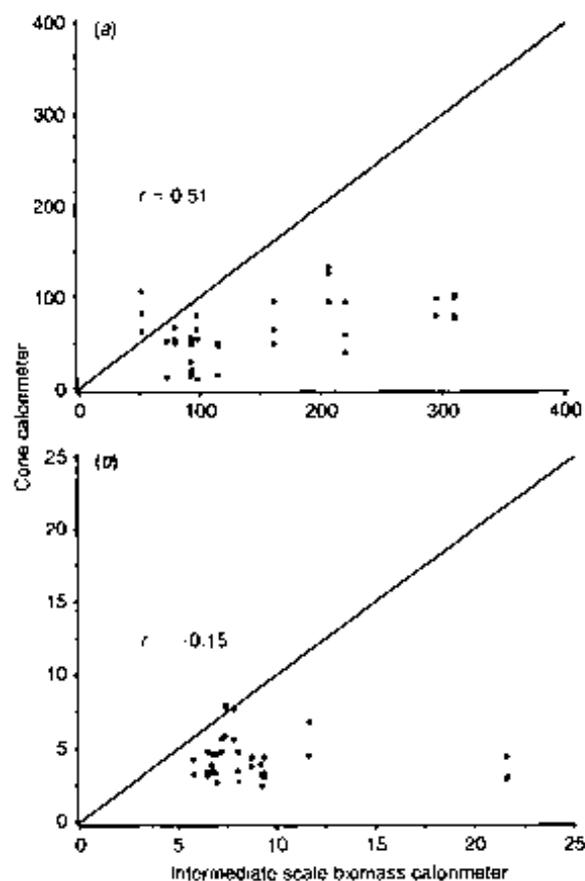
Fig. 11. Correlations of the combustion characteristics measured by a cone calorimeter and an intermediate scale biomass calorimeter. (a) Normalized peak heat release rate ( $\text{kW m}^{-2}$ ); and (b) effective heat of combustion ( $\text{MJ kg}^{-1}$ ).
