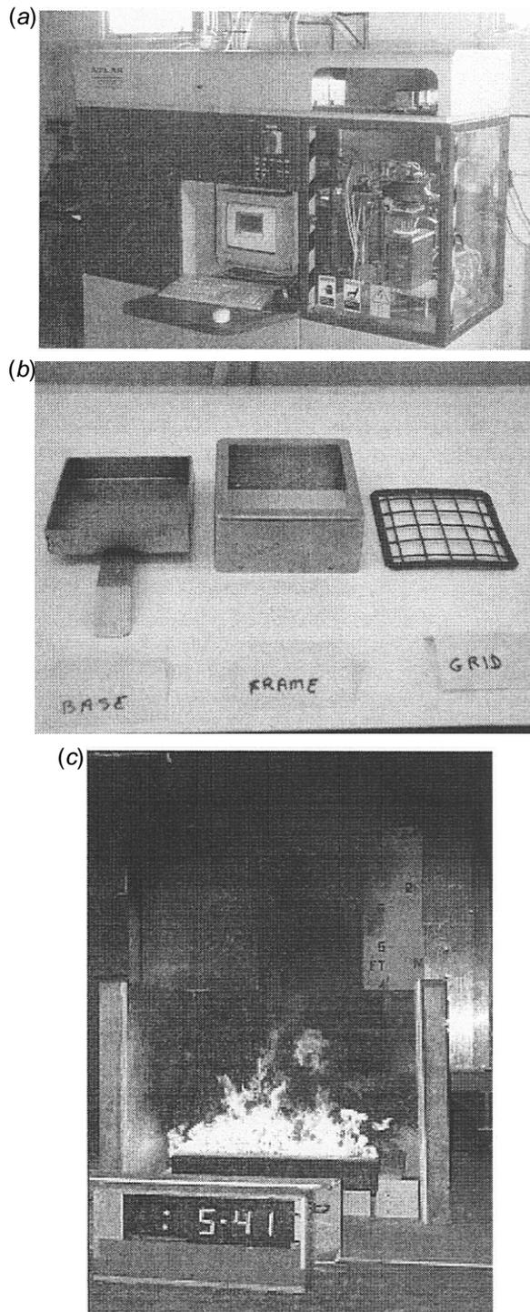
**Fig. 2.** (a) Cone calorimeter used to measure combustion characteristics of various vegetation specimens, (b) specimen holder with retainer frame and grid used by cone calorimeter and (c) intermediate scale biomass calorimeter used to measure combustion characteristics of small shrubs.
