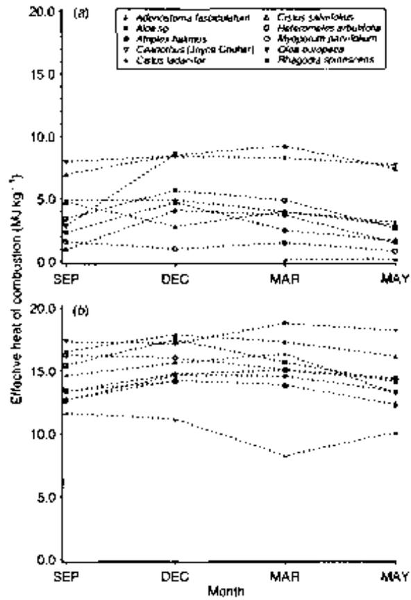
Fig. 6. Mean effective heat of combustion (EHOC) for (a) green and (b) oven-dry samples of ornamental vegetation in southern California. The EHOC was determined using 25 kW m<sup>-2</sup> flux in a cone calorimeter.
