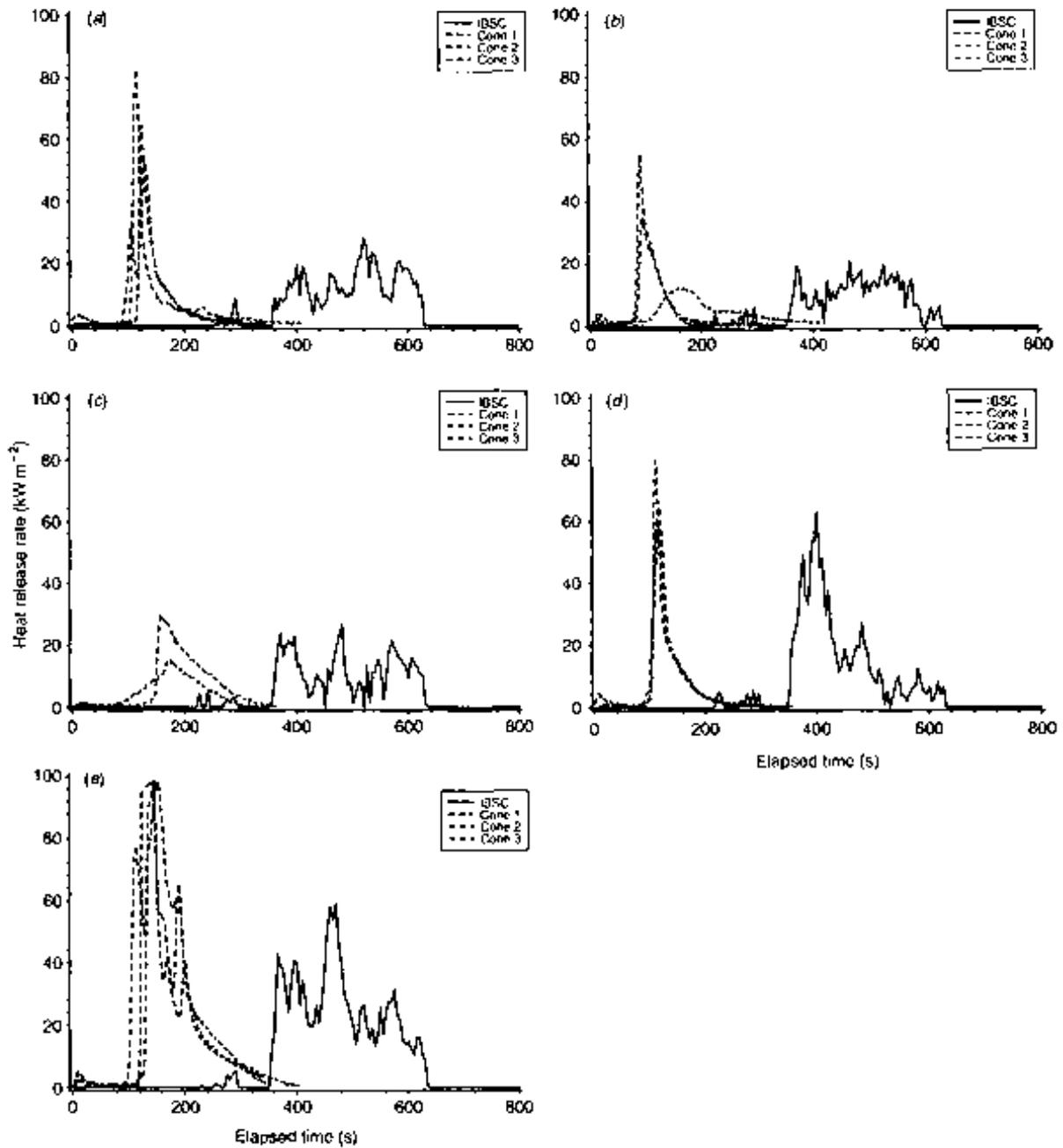
**Fig. 10.** Heat release rates measured by a cone calorimeter and an intermediate scale biomass calorimeter for five plant species used to landscape yards in California. (a) *Atriplex lentiformis*; (b) *Ceanothus impressus*; (c) *Cistus salvifolius*; (d) *Rhagodia spinescens*; and (e) *Rosmarinus officinalis*.
