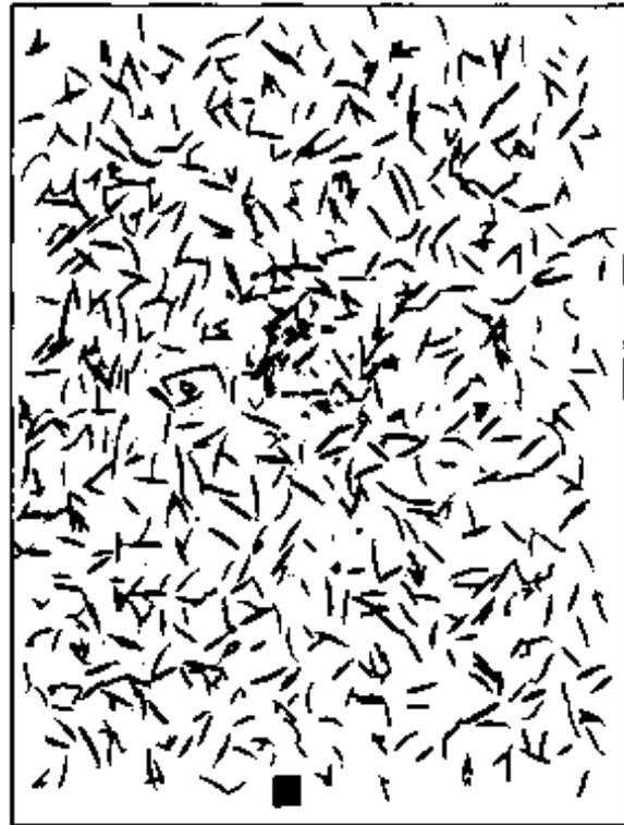
**Fig. 1.** Scanned image of *Rosmarinus officinalis* used to determine surface area-to-volume ratio at University of California Forest Products Laboratory. The square in the lower portion of the figure is 1-cm<sup>2</sup> calibration image.
