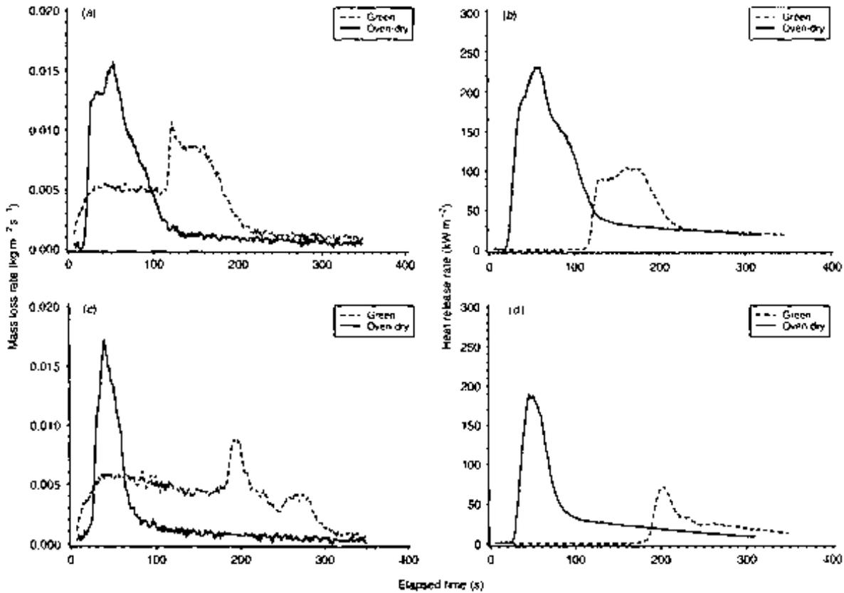
**Fig. 4.** Mass loss rates and heat release rates measured in a cone calorimeter for green and oven-dry samples of (a,b) chamise (*Adenostoma fasciculatum*) and (c,d) saltbush (*Atriplex halimus*).
