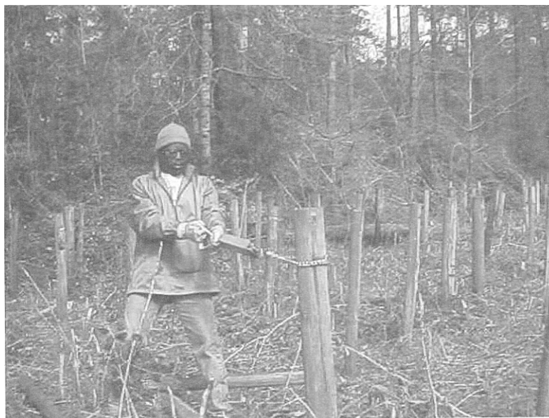
Example of 50 lb Pull test
