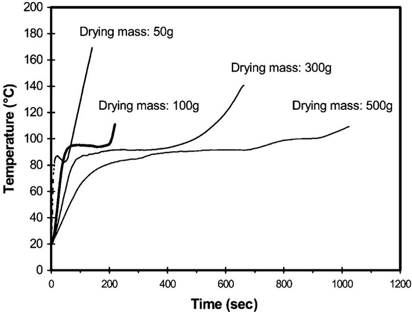
Figure 4. Temperature changes during microwave drying under 687 W power input for different drying weights.
