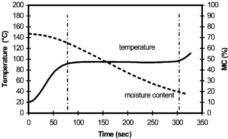
Figure 2. Typical temperature and MC changes during microwave drying (power input = 687 W and drying mass = 100 g).
