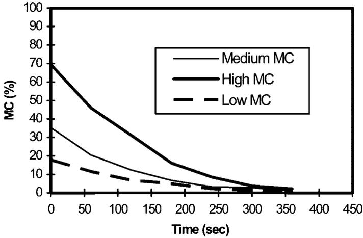
Figure 6. The moisture changes of the three different groups during microwave drying.
