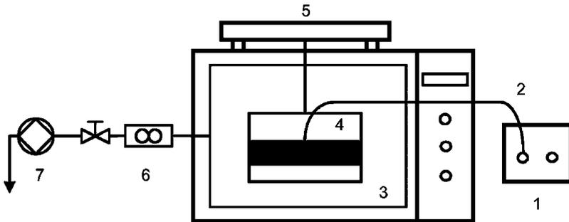
*Figure 1.* Schematic diagram of the test equipment: 1) Fiber optical data logger, 2) fiber optical temperature sensor, 3) microwave oven, 4) sample container, 5) electric balance, 6) flow meter, 7) vacuum pump.
