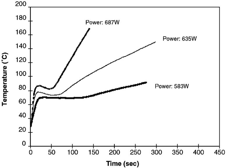
**Figure 3.** Temperature changes during microwave drying of 50 g of wood strands at different power inputs.
