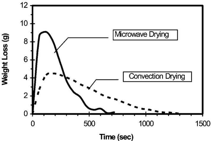
Figure 9. Comparison of weight loss for the two drying methods.
