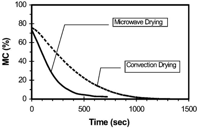
Figure 8. Comparison of moisture change rates for the two drying methods.
