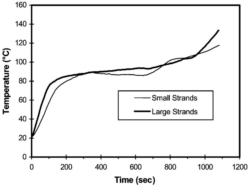
*Figure 5.* The effect of strand geometry on temperature changes during microwave drying.
