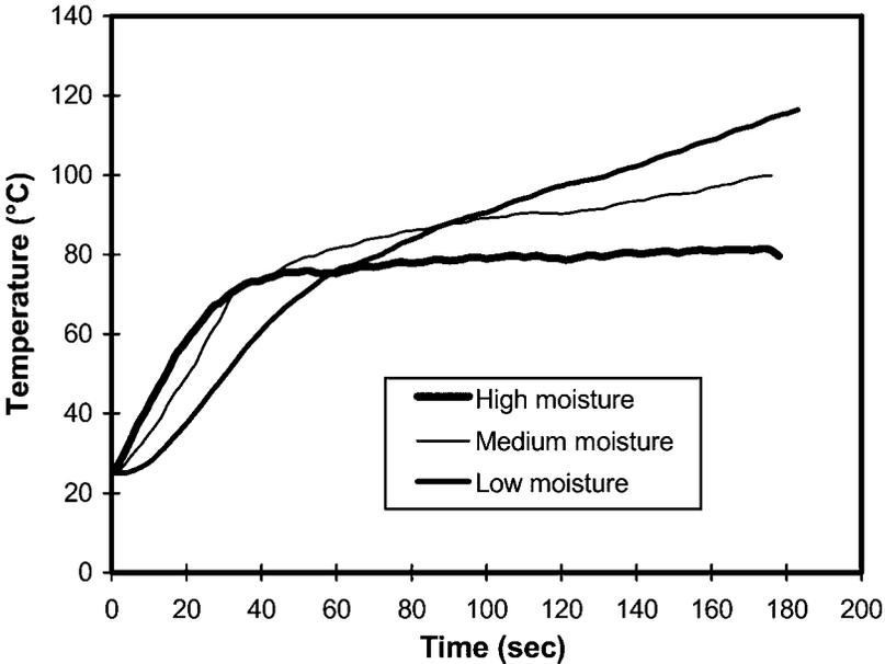
Figure 7. The effect of initial MCs on temperature changes during microwave drying.
