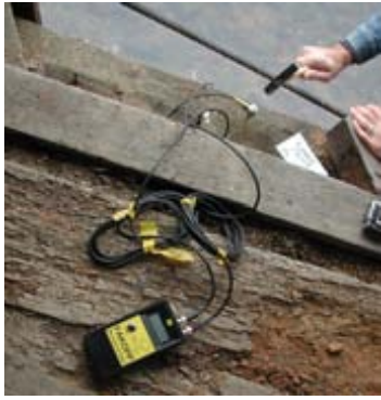
Figure 8 - Using a stress-wave timer to detect interior decay in a lower chord member”
