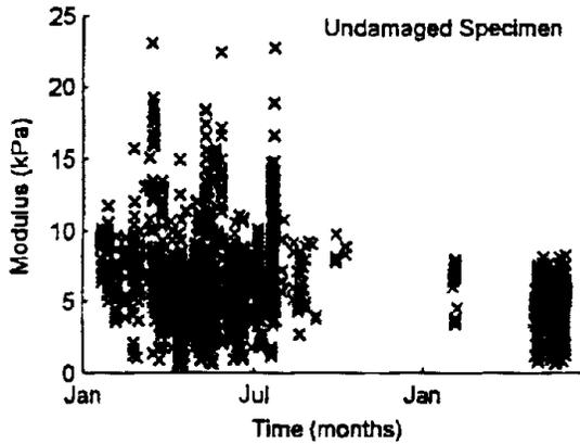
Figure 29. Approximated elastic modulus ( $R^2 > 99\%$ ,  $w = 4$  fitting method) for an undamaged specimen.
