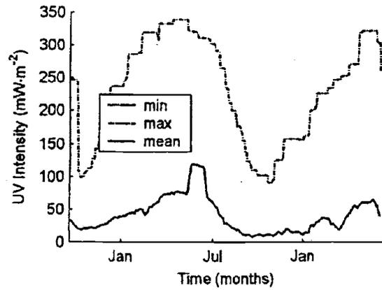
Figure 21. Yearly histogram of UV irradiance at 323.45 nm. Maximum, minimum, and mean values are shown for week-long intervals. (Minimum value lies along the 0 axis.)
