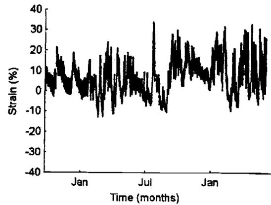
Figure 24. Strain as a function of time on CS-type apparatus for a 20-month exposure period.
