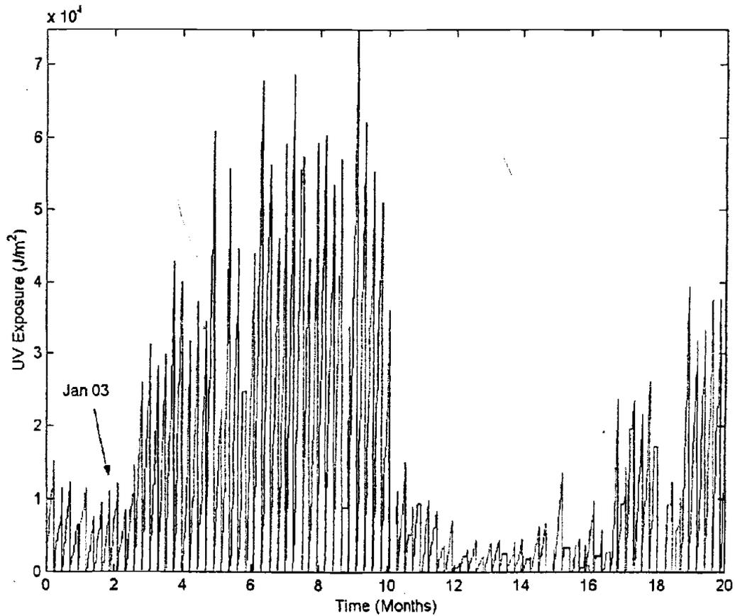
Figure 22. Weekly totals of spectral radiant exposure ( $J/m^2$ ) at 340 nm.
