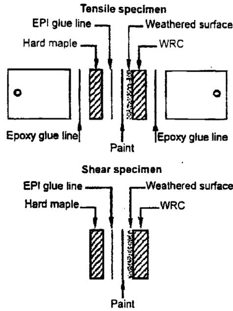
Figure 1. Expanded view of tensile and shear specimens showing interphases (ML86-5258)
