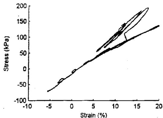
Figure 34. Sudden failure of a specimen. The change in slope occurred on 2004-05-12 at 14:27 CST. Ambient temperature was 19°C. Ambient RH was 45%. It had rained the previous day. The wood engine in the CS apparatus was in a drying cycle, which placed tension on the specimen.
