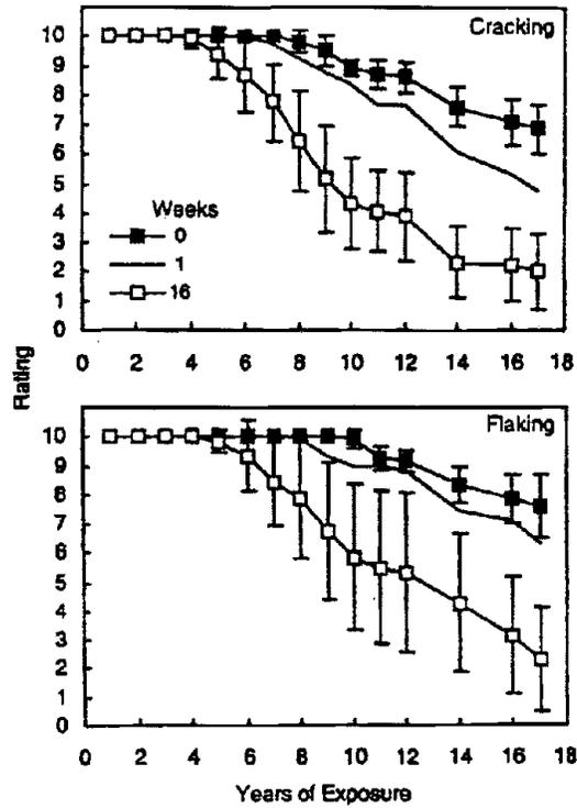
Figure 14. Paint evaluations for cracking and flaking during 17 years of outdoor exposure for specimens painted with one coat of latex primer and one coat of acrylic latex topcoat (latex/latex). The data points are the average of 12 observations, and the bars give the standard deviation.
