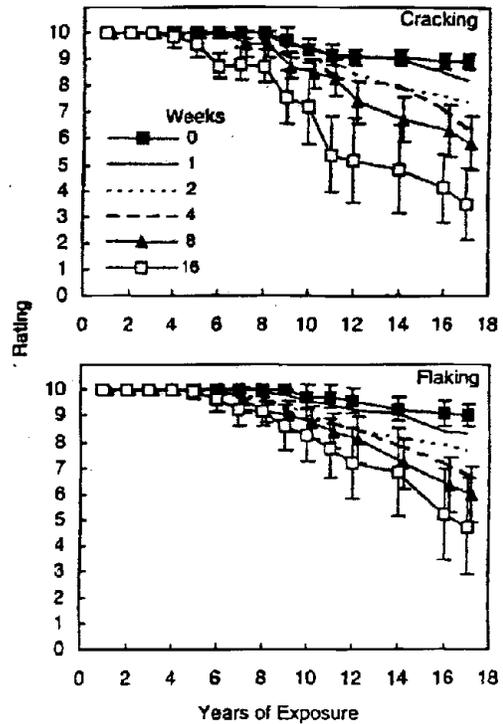
Figure 9. Paint evaluations for cracking and flaking during 17 years of outdoor exposure for specimens painted with a solventborne water-repellent preservative, one coat of alkyd-oil primer, and one coat of acrylic latex topcoat (WRP/alkyd/latex). The data points are the average of 12 observations, and the bars give the standard deviation.
