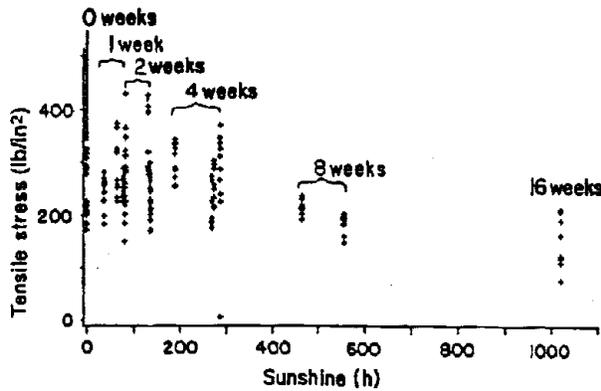
Figure 5. Ultimate tensile stress compared with sunlight exposure time of acrylic latex primer on western redcedar. All adhesive failures and cohesive wood failures are shown (1 kb/in<sup>2</sup> = 6.9 kPa). (ML 86 5259)
