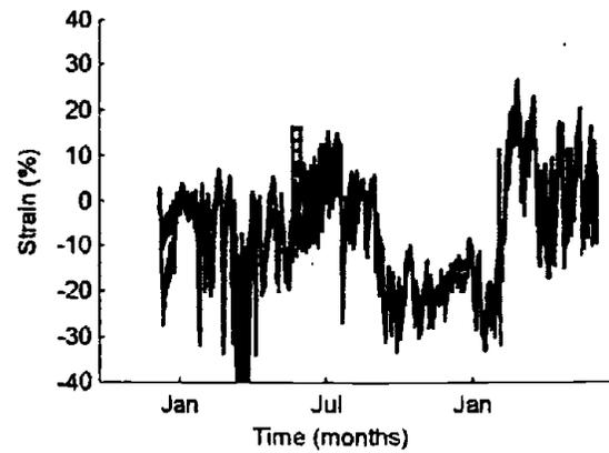
Figure 26. Strain as a function of time on TS-type apparatus for a 16-month exposure period.
