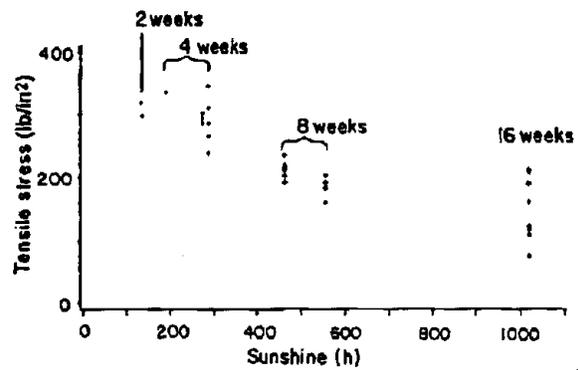
Figure 6. Ultimate tensile stress compared with sunlight exposure time of acrylic latex primer on western redcedar. Only primer/wood interphase failures are shown (1 lb/in<sup>2</sup> = 6.9 kPa). (ML 86 5259)
