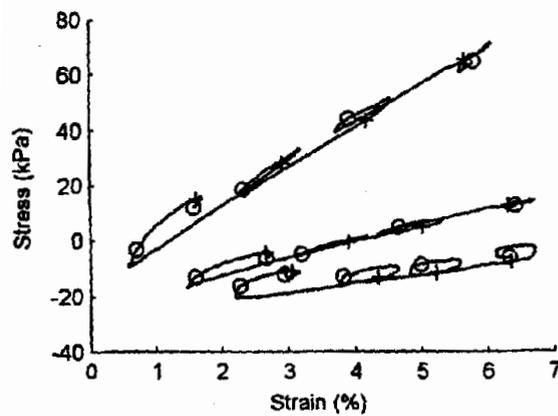
Figure 17. Stress-strain plot highlighting temperature-induced looping phenomenon. Three different sealant formulations are shown.
