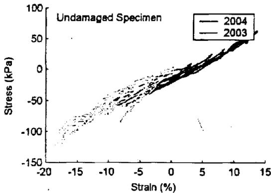
Figure 31. Comparison of stress-strain behavior of an undamaged specimen for 3-month periods in 2003 and 2004.
