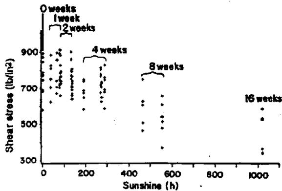
Figure 8. Ultimate shear stress compared with sunlight exposure time of acrylic latex primer on western redcedar. All adhesive failures and cohesive wood failures are shown (1 lb/in<sup>2</sup> = 6.9 kPa). (ML 86 5261)
