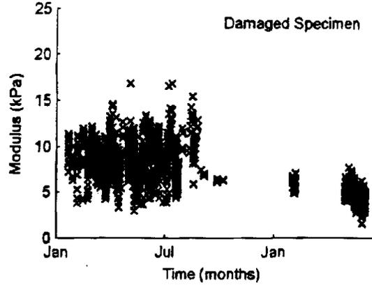
Figure 30. Approximated elastic modulus (using the  $R^2 > 99\%$ ,  $w = 4$  fitting method) for a degraded specimen.
