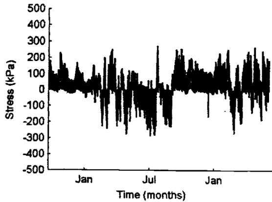
Figure 23. Stress as a function of time on CS-type apparatus for a 20-month exposure period.
