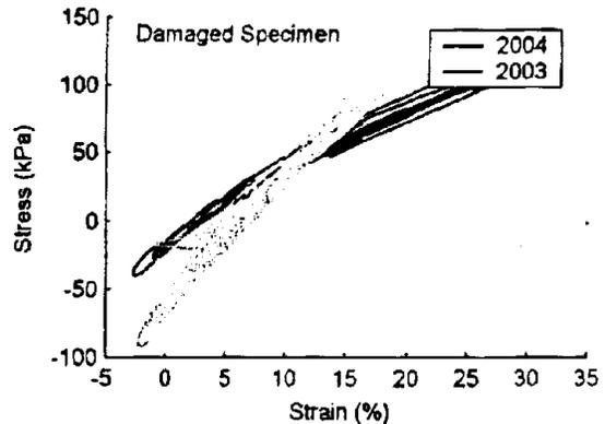
Figure 32. Comparison of stress-strain behavior of a degraded specimen for 3-month periods in 2003 and 2004.
