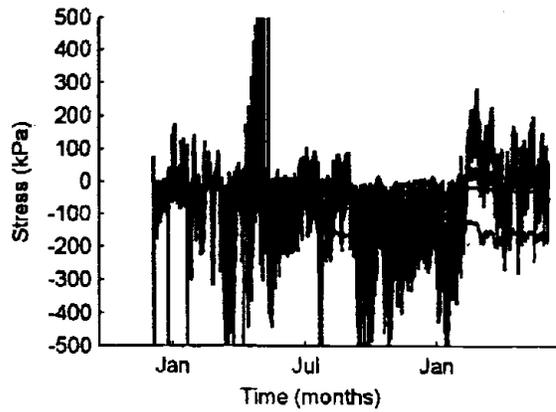
Figure 25. Stress as a function of time on TS-type apparatus for a 16-month exposure period.
