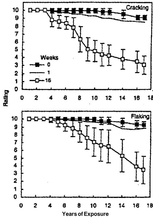
Figure 12. Paint evaluations for cracking and flaking during 17 years of outdoor exposure for specimens painted with one coat of alkyd-oil primer and one coat of acrylic latex topcoat (alkyd/latex). The data points are the average of 12 observations, and the bars give the standard deviation.
