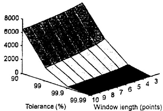
Figure 28. Analysis of data breakdown procedure. when selecting a fit to a given  $R^2$  tolerance (on the  $x$  axis) using a given window length (on they axis), the  $z$  axis gives the number of points obtained.
