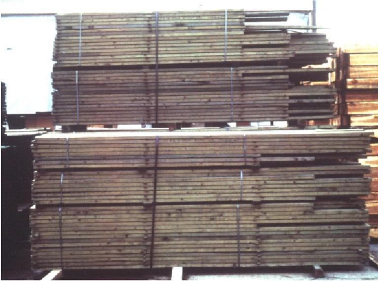
**Figure 4** Lumber treated with copper citrate (CC).
