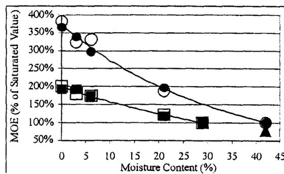
Figure 1. (Left) Spruce tangential and radial MOE as a function of moisture content % of MOE at saturation. Open and closed circles, tangential and radial measurements of *C. subvermispota* treated material. Open and closed squares, tangential and radial measurements of control material. Triangle represents the extrapolation of the untreated control to the moisture content of biopulped material (42%).
