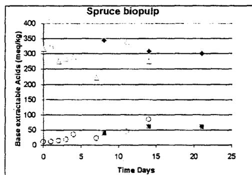
Figure 2. (Right) Spruce biopulp analyzed for base extractable acids. Triangles and diamonds, acetate from *C. subvermispota* and *P. chrysosporium* respectively. Circles and squares, oxalate from *C. subvermispota* and *P. chrysosporium* respectively.
