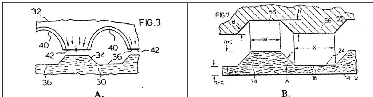
Figure 5 - Patent 4,904,517 (A.) selectively places additional flakes in areas for ribbed sections and (B.) using machined platens to produce a panel with one ribbed side and one flat side.
