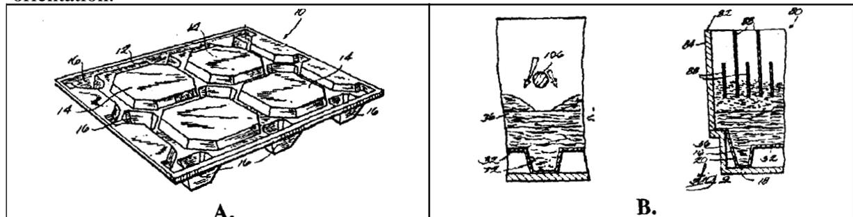
Figure 6 - Patent 5,142,994 consolidates wood flakes and particles into a pallet (A.). Flake and Particle distribution and orientation methods (B.) are also described.
