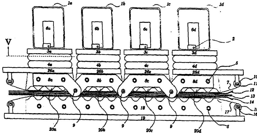
Figure 2 - Patents 4,816,103 and 4,943,339 use an articulated hinged batch press to corrugate wood veneer.
