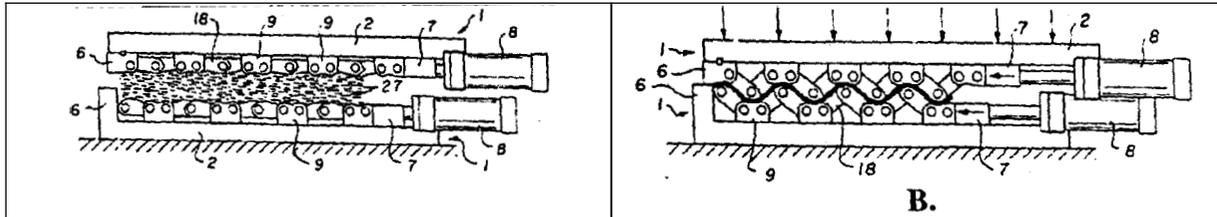
Figure 4 - Patents 4,616,991; 4,675,138; 5,047,280; and 5,443,891 consolidates a planer mat of wood wafers (A.) using movable platens (B.) to produce a corrugated structure.
