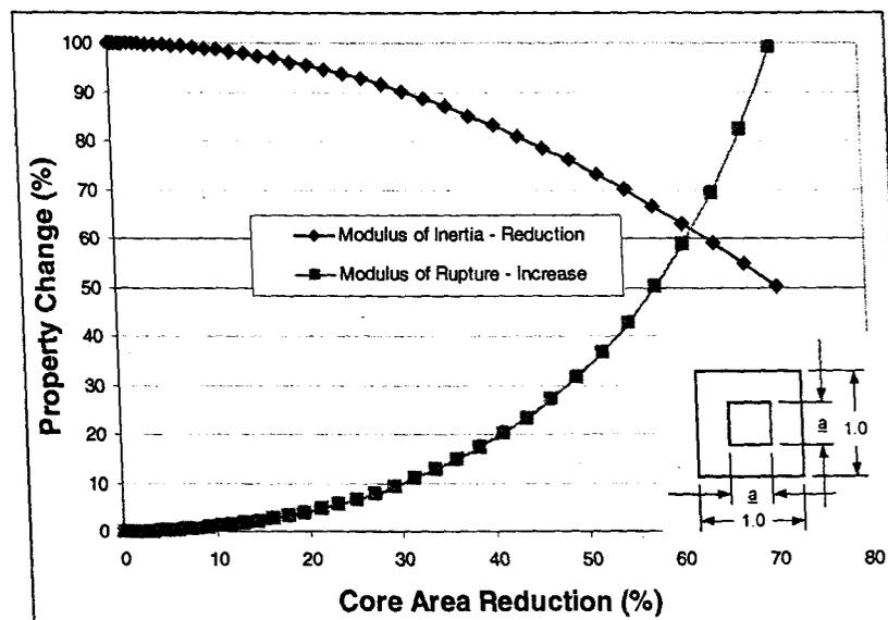
Figure 1 - Effect of reduction of the core area ( $a$  by  $a$ ) on the theoretical beam's area moment of inertia and modulus of rupture at the surface of the beam.
