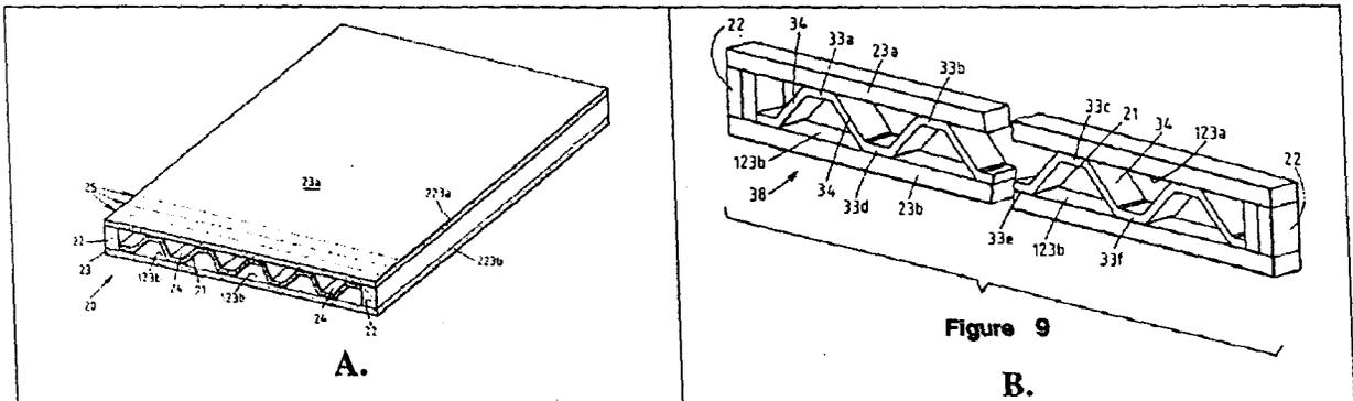
Figure 3 - Patent 6,511,567; 6,541,097; and 6,773,791 combines a uniform dense core made from flakes with face and end pieces to construct a structural lumber product.
