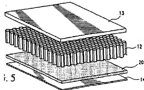
**Figure 11 –Patent 6,711,872 shows common light-weight gypsum panel with the core made from honeycomb paper.**
