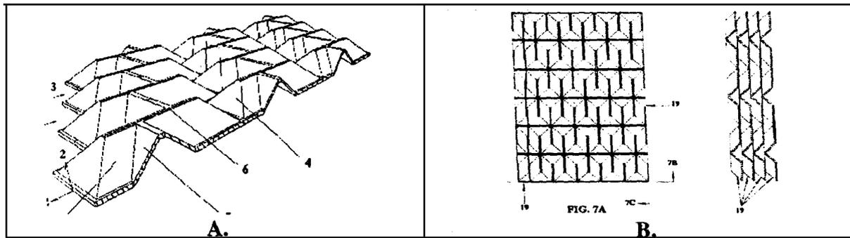
Figure 9 - Patent 5,900,304 and 6,451,235 uses a wet-slurry process to produce a 3D structural panels (A.) that have unique two-direction pyramid like rib structure and are stackable (B.).
