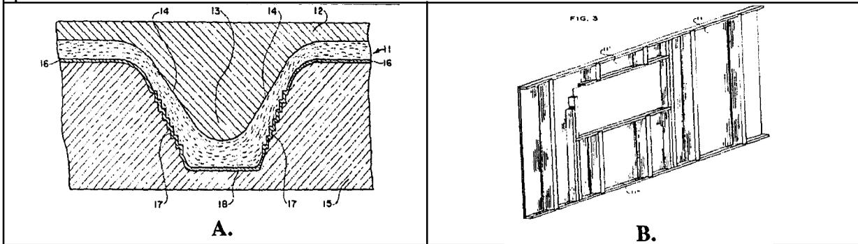
Figure 7 - Patents 4,061,813 consolidates wood flakes or particles (A.) to form a complete sheathing and framing wall system.
