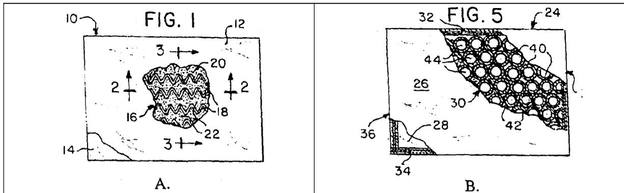
Figure 13. - Patent 5,738,924 shows the top view of two structural core embodiments: (A.) corrugated material on edge; and (B.) bamboo or tubes of some fabrication.
