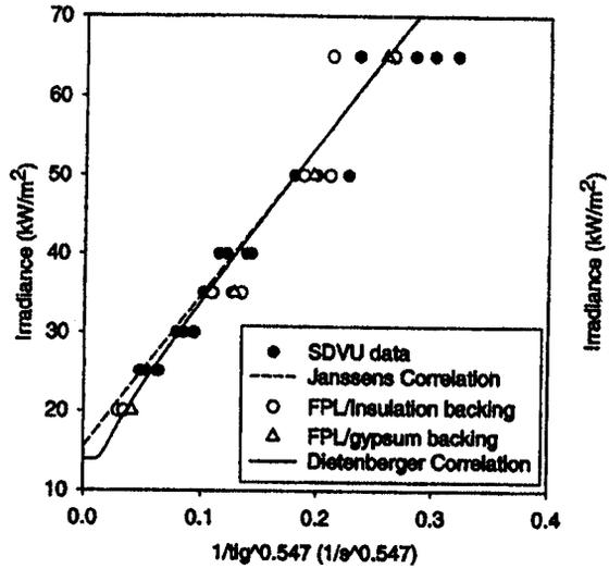
Figure 6. Correlation to piloted ignition data of Gypsum X (ISO 1)
