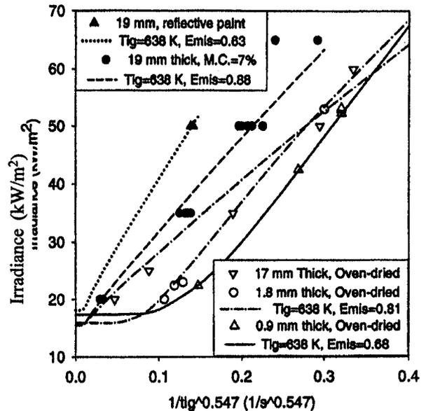
Figure 1. Prediction of redwood piloted ignition with varying irradiance, thickness, moisture content, and surface emissivity using Dietenberger's correlation
