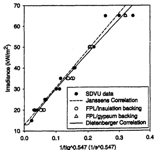
Figure 4. Correlation to piloted ignition data of Douglas-fir plywood (ASTM) (ISO 5)
