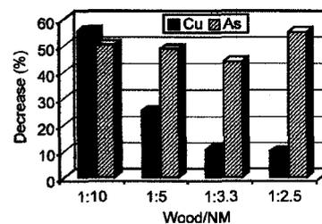
Fig. 2. Percentage decrease of copper and arsenic in CCA-treated particles following exposure to *B. licheniformis* in culture with varying ratios of wood to nutrient medium (NM). *B. licheniformis* alone does not remove chromium from CCA-treated wood.
