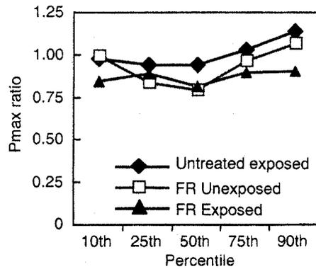
FIG. 3—Ratio of maximum load capacity ( $P_{max}$ ) of treated and exposed 2 by 4 southern pine lumber and  $P_{max}$  of matched untreated, unexposed controls across distribution for each treatment-high-temperature exposure group.
