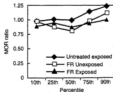
FIG. 2—Ratio of modulus of rupture (*MOR*) of treated and exposed 2 by 4 southern pine lumber and *MOR* of matched untreated, unexposed controls across distribution for each treatment-high-temperature exposure group.
