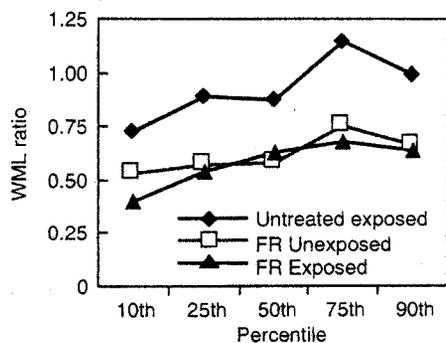
FIG. 4—Ratio of work to maximum load (WML) of treated and exposed 2 by 4 southern pine lumber and WML of matched untreated, unexposed controls across distribution for each treatment-high-temperature exposure group.
