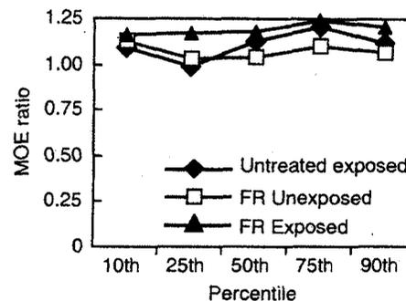
FIG. 1—Ratio of modulus of elasticity (*MOE*) of treated and exposed 2 by 4 southern pine lumber and *MOE* of matched untreated, unexposed controls across distribution for each treatment-temperature exposure group.
