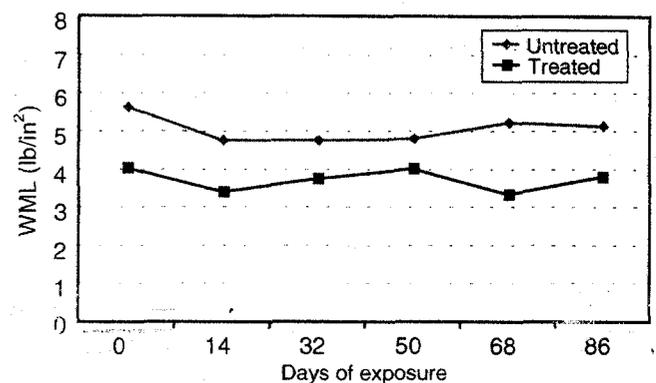
FIG. 3—Work to maximum load of FR-treated and untreated Douglas-fir plywood. 1 in. ·lb/in. <sup>3</sup> = 6.895 kJ/m<sup>3</sup>
