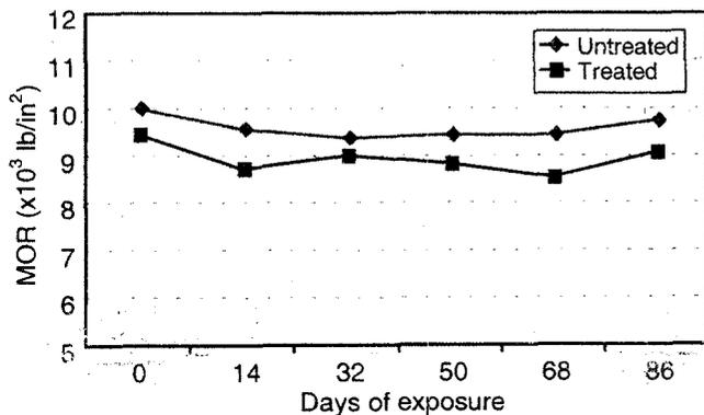
FIG. 1—Modulus of rupture of FR-treated and untreated Douglas-fir plywood 1 lb/in. <sup>2</sup> = 6.895 kPa.
