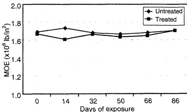
FIG. 2—Modulus of elasticity of FR-treated and untreated Douglas-fir plywood. lb/in. <sup>2</sup> = 6.895 kPa.
