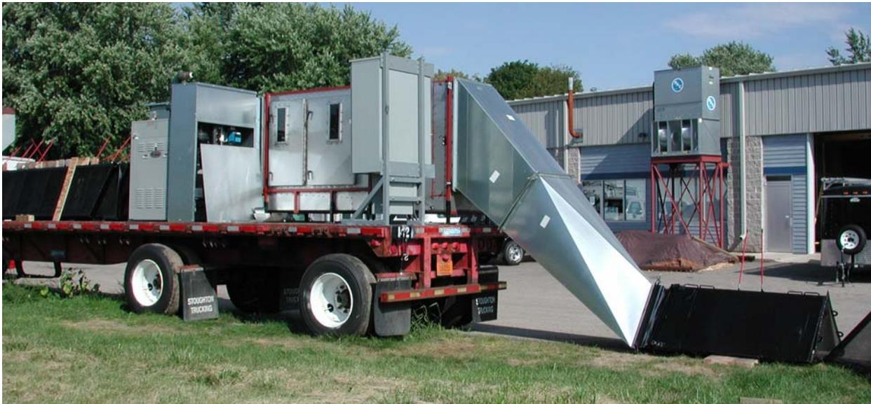
Figure 5. Ventilation/conditioning equipment trailer.
