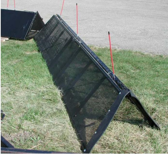
Figure 4. Section of portable under-pile ventilation tunnel.
