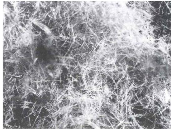
FIG. 4. Refined 40-mesh wood fiber.
