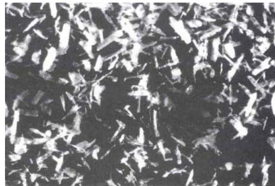
FIG. 2. Screened 70-mesh wood flour.
