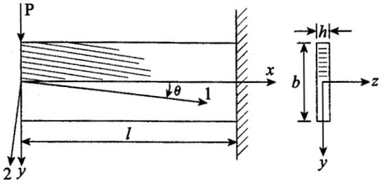
FIG. 1. Orthotropic cantilever subjected to single load.  $x$  and  $y$  are geometrical axes; 1 and 2 are material axes.
