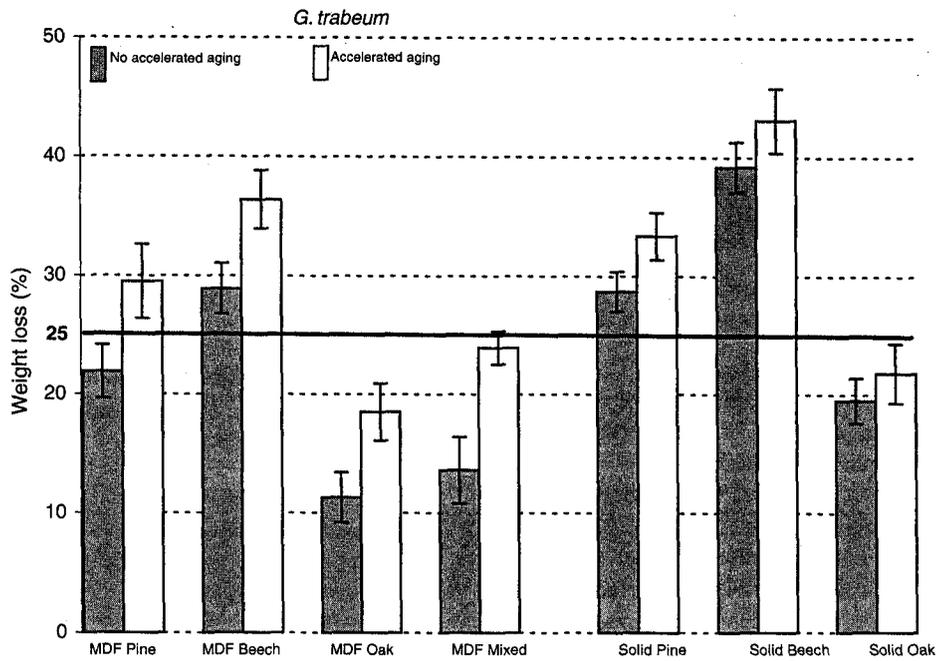
Fig. 2. Weight losses in MDF and solid wood specimens after 12-week exposure against *G. trabeum*. Each value represents the means of 12 replications. Specimen with weight loss of < 25% is classified resistant.
