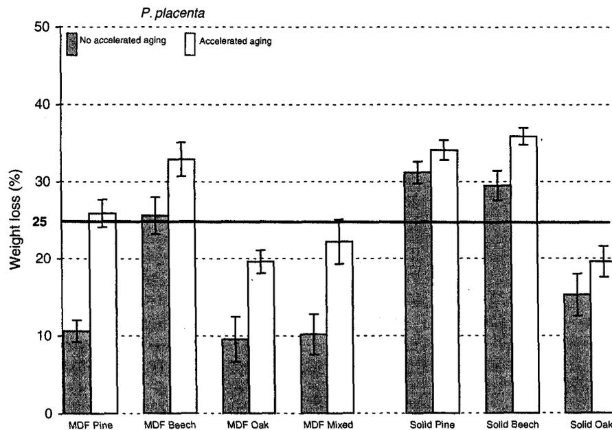
Fig. 3. Weight losses in MDF and solid wood specimens after 12-week exposures against *P. placenta*. Each value represents the means of 12 replications. Specimen with weight loss of < 25% is classified resistant.
