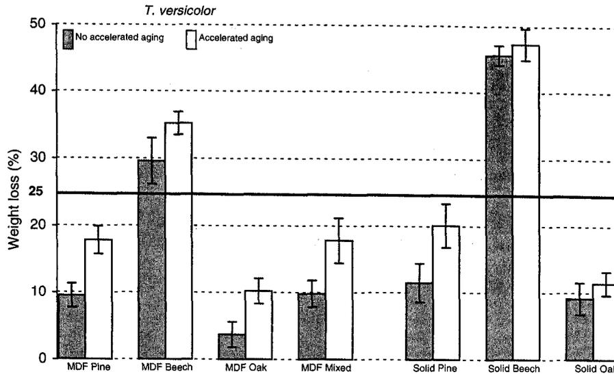
Fig. 4. Weight losses in MDF and solid wood specimens after 12-week exposure against *T. versicolor*. Each value represents the means of 12 replications. Specimen with weight loss of < 25% is classified resistant.
