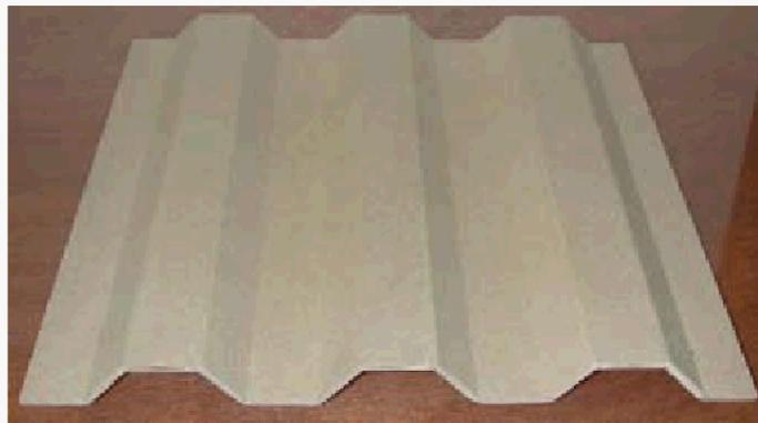
*Fig.1 preliminary design of a uniaxial core made from fiberized fibers from small diameter tree tops*
