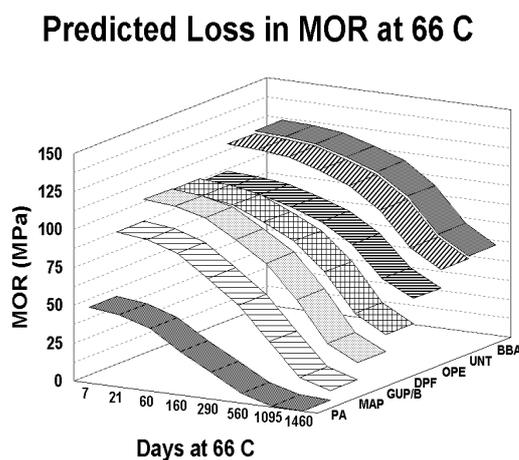
**Figure 3. Predicted bending strength loss with time of exposure to 66°C (Lebow & Winandy 1999). (PA phosphoric acid, MAP monoammonium phosphate, GUP/B guanylurea phosphate/boric acid, DPF dicyandiamide-PA-formaldehyde, OPE organophosphonate ester, UNT untreated, BBA borax/boric acid).**
