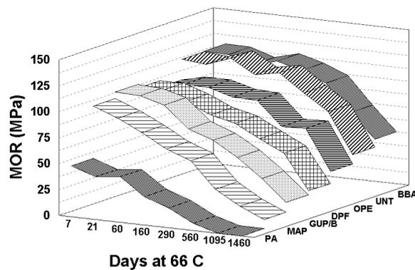
**Figure 2. Experimentally measured bending strength loss with time of exposure to 66°C (Winandy 1995, Lebow & Winandy 1999) (PA phosphoric acid, MAP monoammonium phosphate, GUP/B guanlyurea phosphate/boric acid, DPF dicyandiamide-PA-formaldehyde, OPE organophosphonate ester, UNT untreated, BBA borax/boric acid).**
