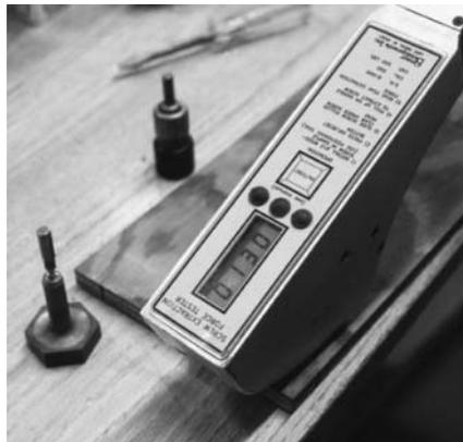
**Figure 5. Screw-pull test using hand-held load cell.**
