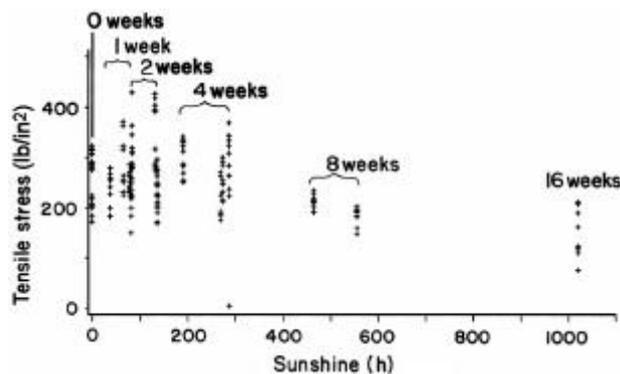
**Figure 2. Ultimate tensile stress compared with sunlight exposure time of acrylic latex primer on WRC. All adhesive failures and cohesive wood failures are shown (1 lb/in<sup>2</sup> = 6.9 kPa) (ML86 5259).**
