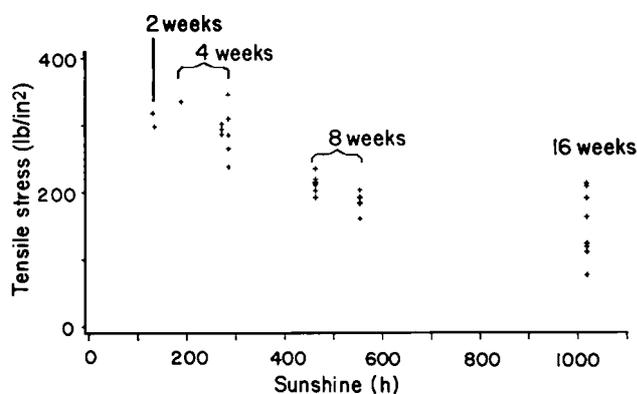
**Figure 3. Ultimate tensile stress compared with sunlight exposure time of acrylic latex primer on WRC. Only primer/wood interphase failures are shown (1 lb/in<sup>2</sup> = 6.9 kPa) (ML86 5260).**
