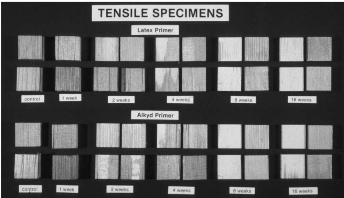
Figure 4. Failure surfaces of representative tensile specimens (M86 0043).
