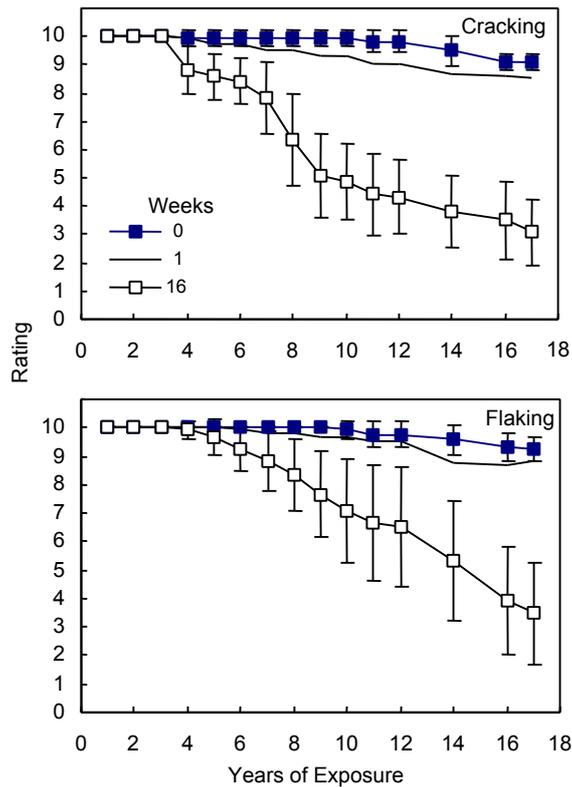
**Figure 9. Paint evaluations for cracking and flaking during 17 years of outdoor exposure for specimens painted with one coat of alkyd-oil primer and one coat of acrylic latex topcoat (alkyd/latex). The data points are the average of 12 observations, and the bars give the standard deviation.**
