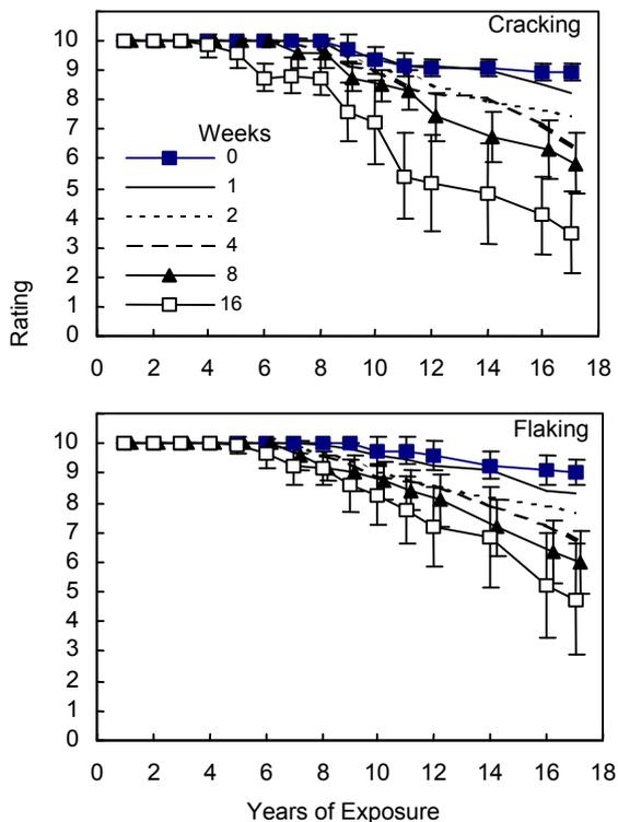
**Figure 6. Paint evaluations for cracking and flaking during 17 years for the paint system of solventborne water-repellent preservative, one coat of alkyd-oil primer, and one coat of acrylic latex topcoat (WRP/alkyd/latex). The data points are the average of 12 observations, and the bars give the standard deviation.**
