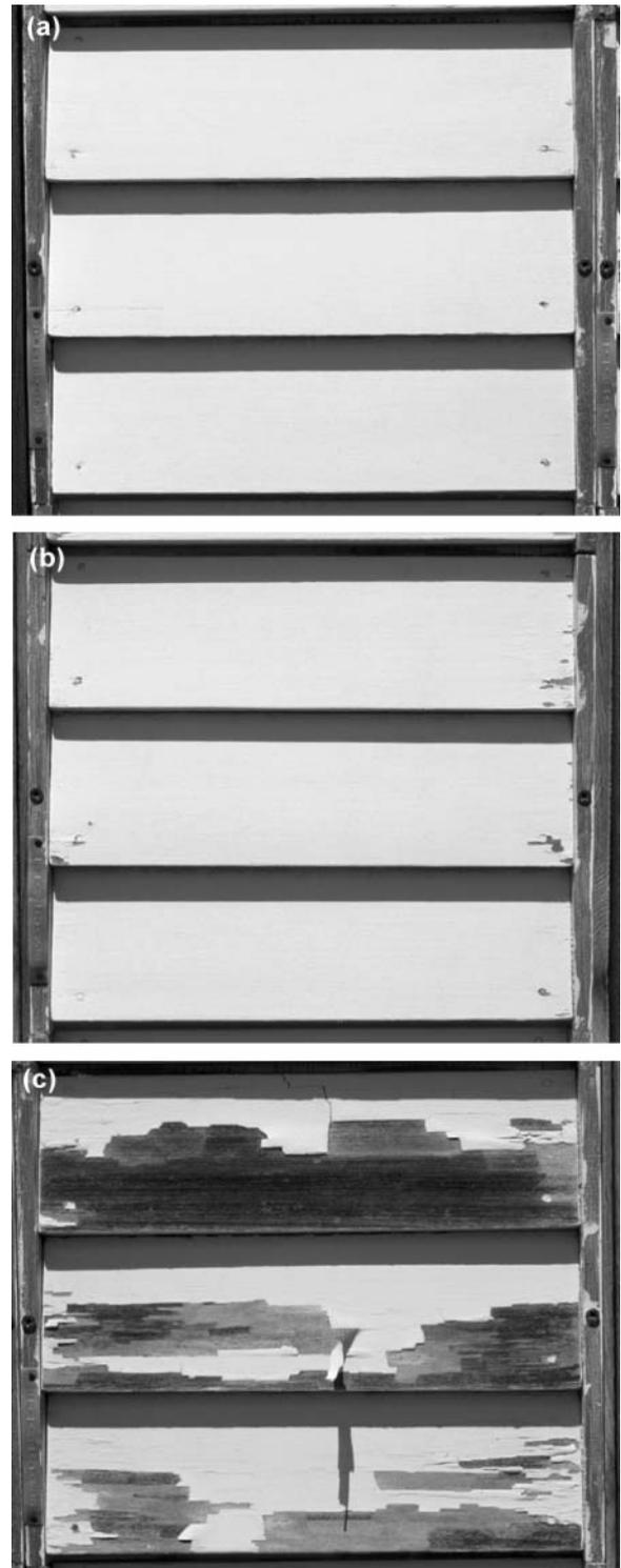
**Figure 10. Examples of panels painted with one coat of alkyd-oil primer and one coat of acrylic latex topcoat (alkyd/latex) after 17 years of outdoor exposure. (a) control, no exposure prior to painting, (b) preweathered 1 week, and (c) preweathered 16 weeks.**
