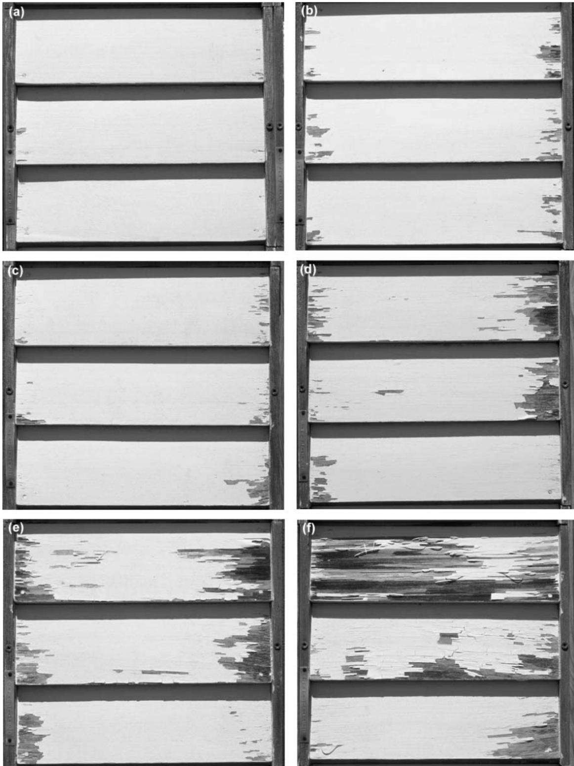
**Figure 8. Examples of panels painted with a solventborne water-repellent preservative, one coat of alkyd-oil primer, and one coat of acrylic latex topcoat (WRP/alkyd/latex) after 17 years of outdoor exposure. (a) control, no exposure prior to painting, (b) preweathered 1 week, (c) preweathered 2 weeks, (d) preweathered 4 weeks, (e) preweathered 8 weeks, and (f) preweathered 16 weeks.**
