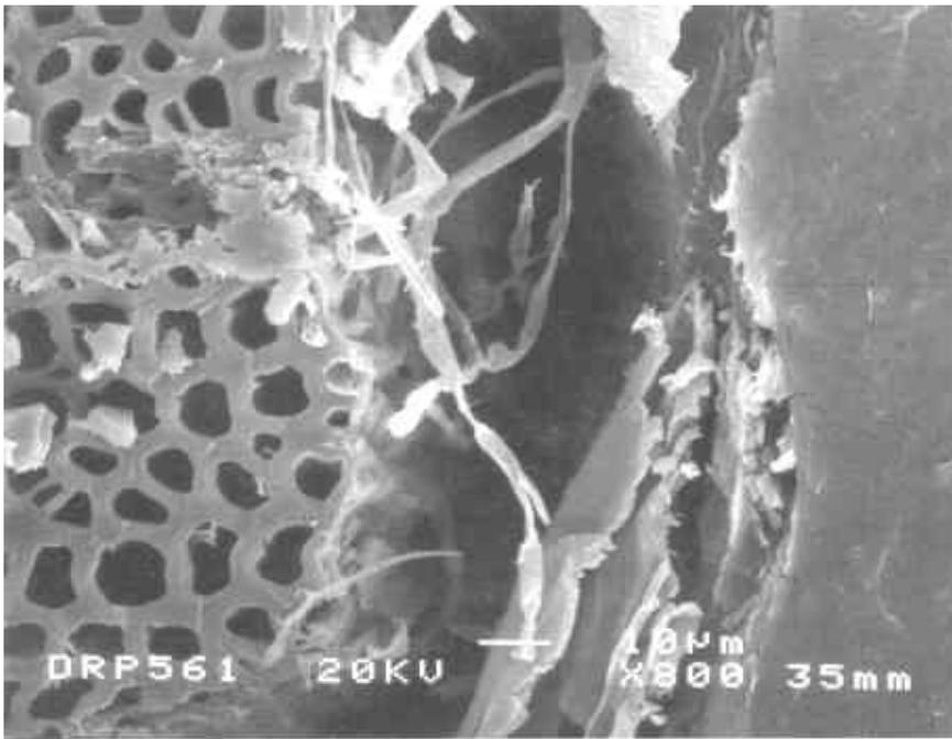
Figure 1.— A scanning electron micrograph of a WPC formulation supporting fungal decay. The mycelium is concentrated in an interfacial gap between the wood and thermoplastic.
