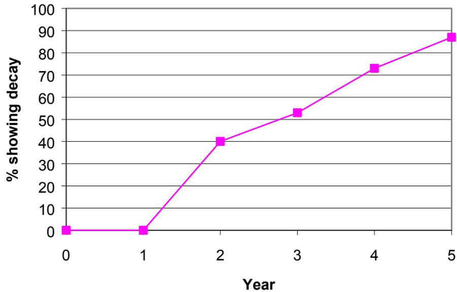
**Figure 1: Percentage of Untreated Pine Sapwood L-Joint Samples Showing Decay When Exposed Outside in Vancouver BC.**
