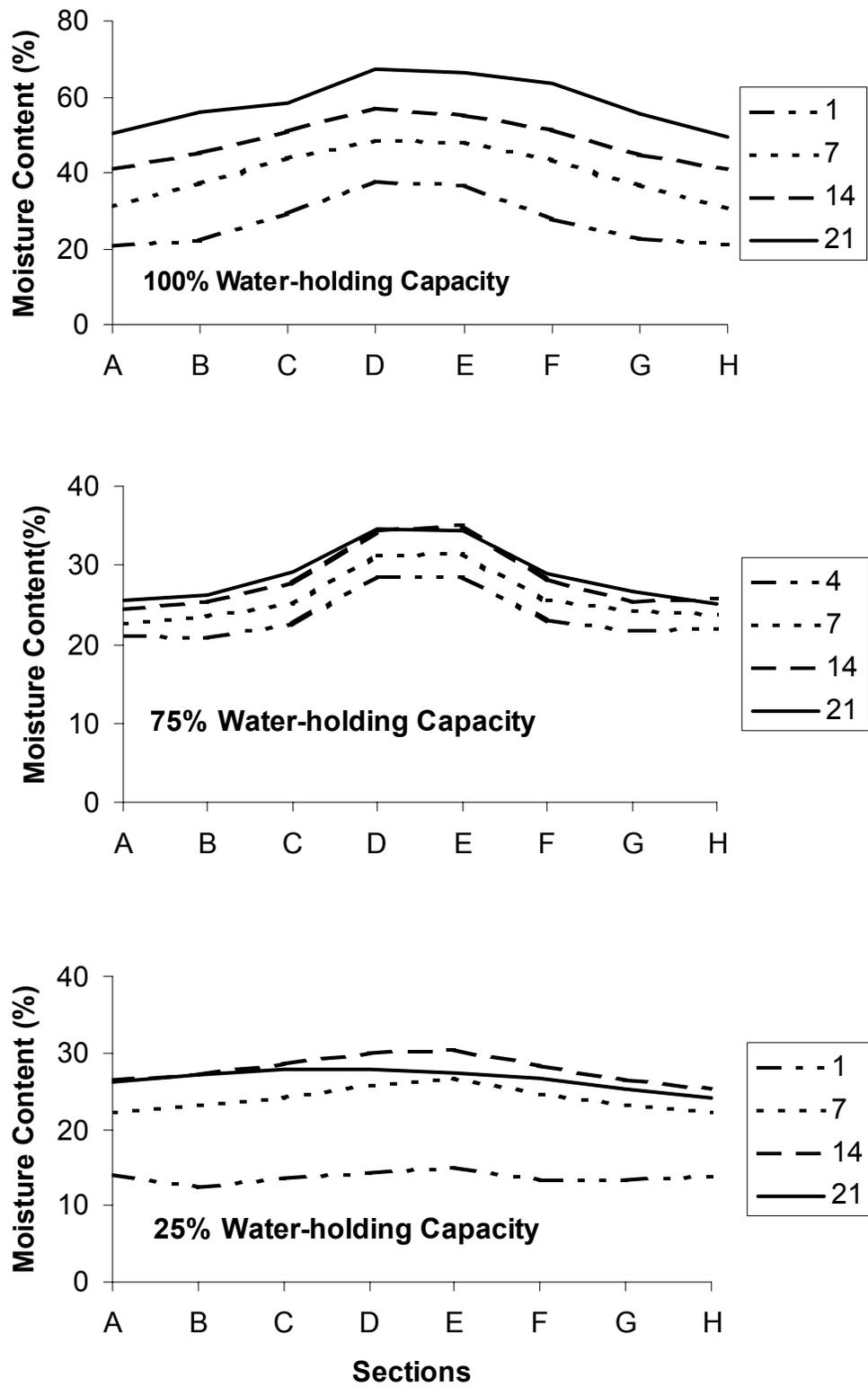
Figure 4: Wood MC From 1 to 21 Days of Exposure at Various Soil Water-Holding Capacities
