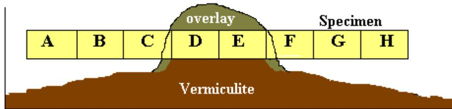
**Figure 2. Diagram Showing Experimental Set Up During Exposure and the Location of Sub-Samples After Removal and Cutting (from Curling et al 2001).**
