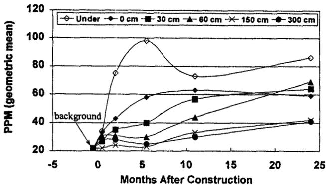
Figure 2.—Copper levels in sediments at six distances from section of boardwalk constructed with CCA-treated wood.
