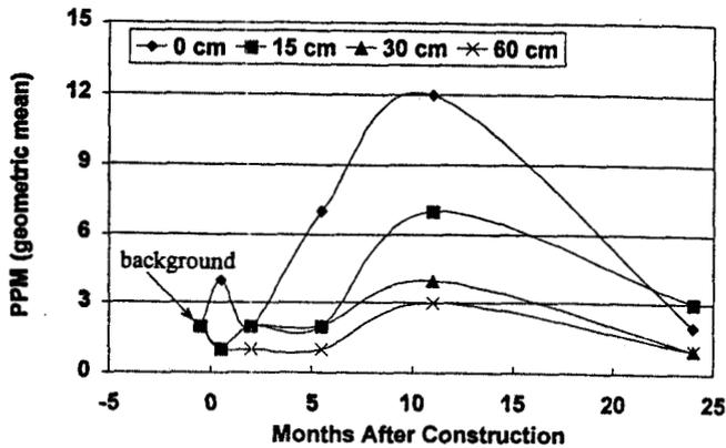
Figure 1.—Arsenic levels in soil at four distances from section of boardwalk constructed with CCA-treated wood.
