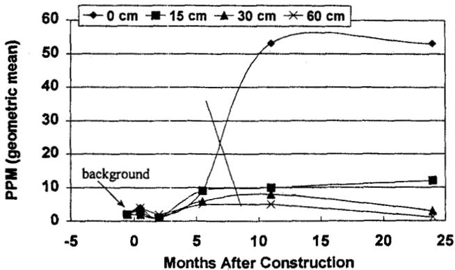
Figure 3.—Arsenic levels in soil at four distances from section of boardwalk constructed with ACZA-treated wood.
