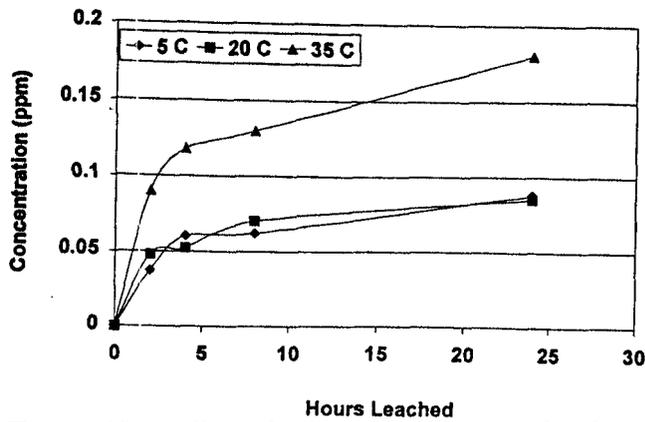
**Figure 19.**—Effect of water temperature on leaching of phenanthrene from creosote-treated lumber submerged in water (without flow).
