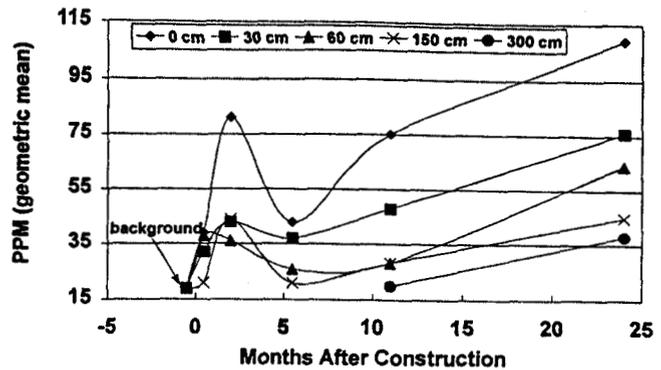
Figure 4.—Copper levels in sediments at six distances from section of boardwalk constructed with ACZA-treated wood.
