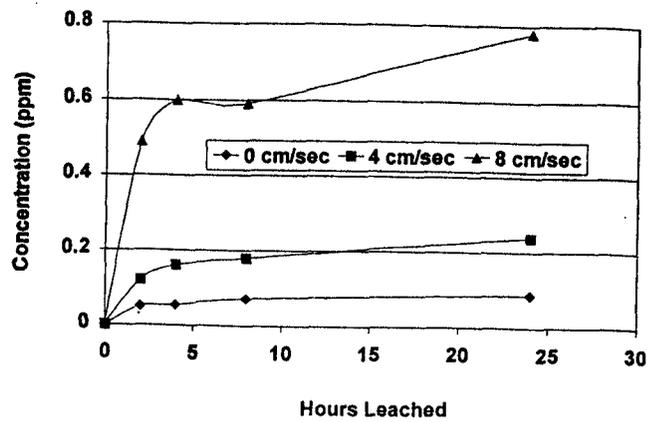
**Figure 20.**—Effect of water flow rate on leaching of phenanthrene from creosote-treated lumber submerged in water at 20°C (68°F).
