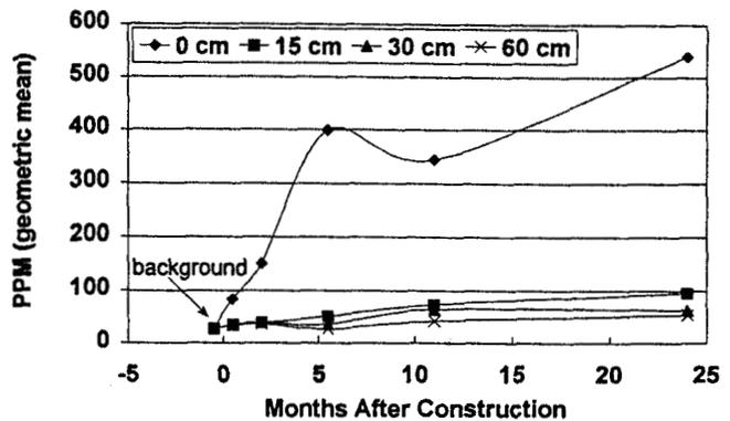
Figure 5.—Copper levels in soil at four distances from section of boardwalk constructed with ACQ-B-treated wood.
