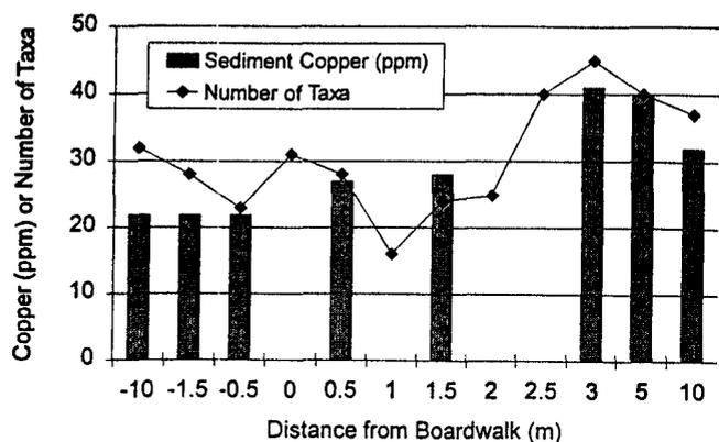
**Figure 7.**—Levels of copper and number of invertebrate taxa in wetland sediments adjacent to the CCA-treated boardwalk 1 year after construction.
