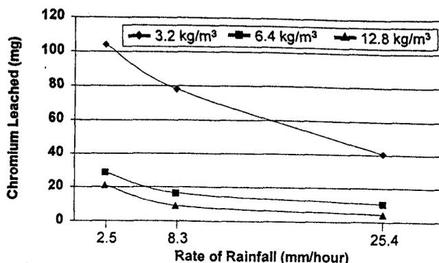
**Figure 15.**—Effect of CCA retention and rate of rainfall on leaching of chromium from decking specimens exposed to artificial rainfall.
