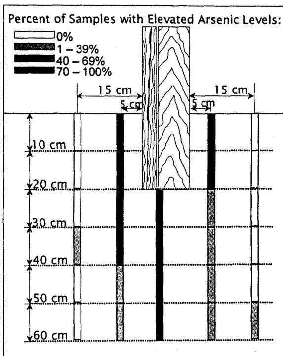
**Figure 11.**—Percent of soil core sample segments with elevated arsenic content at locations beside and below CCA-treated stakes exposed for 22 years in Mississippi.
