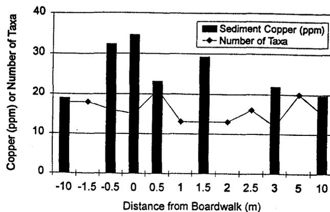
**Figure 8.**—Levels of copper and number of invertebrate taxa in wetland sediments adjacent to the ACZA-treated boardwalk 1 year after construction.
