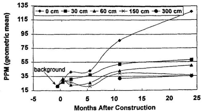
Figure 6.—Copper levels in sediments at four distances from section of boardwalk constructed with ACQ-B-treated wood.
