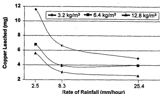
**Figure 14.**—Effect of CCA retention and rate of rainfall on leaching of copper from decking specimens exposed to artificial rainfall.
