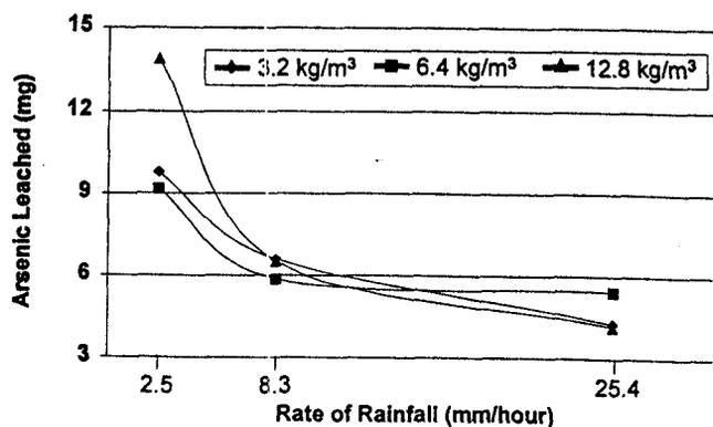
**Figure 13.**—Effect of CCA retention and rate of rainfall on leaching of arsenic from decking specimens exposed to artificial rainfall.
