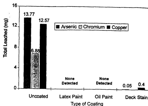
Figure 16.—Effect of coatings on leaching of arsenic, chromium, and copper from CCA-treated decking specimens.
