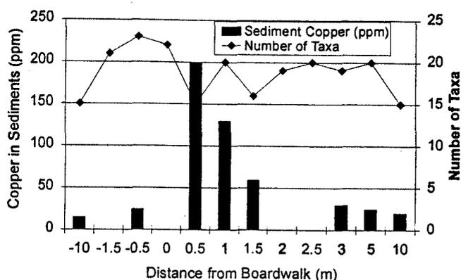
**Figure 9.**—Levels of copper and number of invertebrate taxa in wetland sediments adjacent to the ACQ-B treated boardwalk 1 year after construction.
