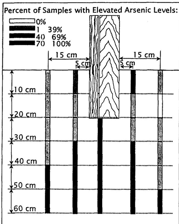
**Figure 12.**—Percent of soil core sample segments with elevated arsenic content at locations beside and below CCA-treated stakes exposed for 22 years in Wisconsin.
