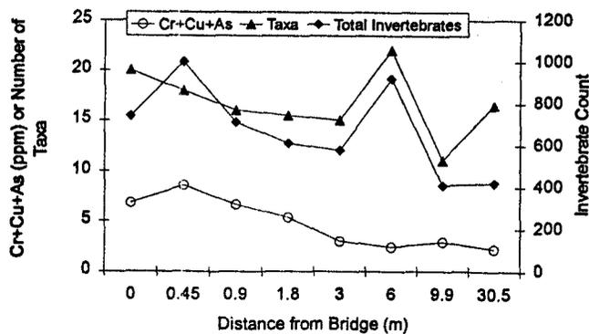
**Figure 10.**—Combined levels of chromium, copper, and arsenic in sediments compared to number of invertebrate taxa and total number of invertebrates adjacent to a CCA-treated bridge.
