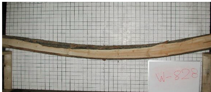
Figure 3. Example of a 6% curve d small tree cut horns-up through a conventional band saw.
