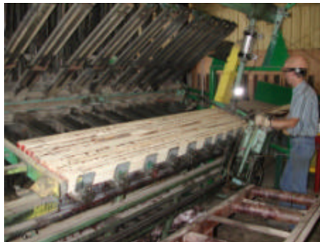
Figure 6. Two beams made from six 2x4s 8 feet long being clamped in a gluing rack.
