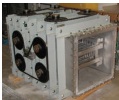
Figure 4. View inside the microwave drying chamber showing the pressing bars that will be used to straighten and hold the curved 2x4s during drying.
