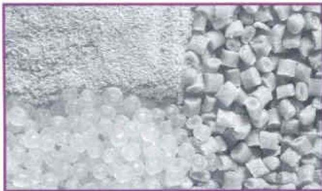
Figure 2. - Compounded pellets (bottom) made from wood (upper right) and plastic (upper left).
