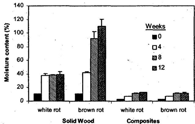
Figure 1—Water sorption of leached solid wood and wood-plastic composites exposed to white-rot (*T. versicolor*) and brown-rot (*G. trabeum*) fungi in soil blocktests.
