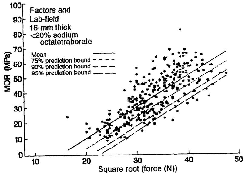
Figure 7. — Mean and lower bounds for predicting bending strength from screw-extraction force measurements on 16-mm-thick, phosphate-treated plywood with  $\leq 20$  percent borate (28).
