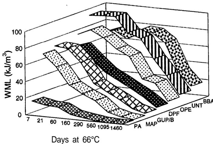
Figure 3.— Predicted change in work to maximum load (WML) over steady-state exposure of up to 4 years at 66°C for untreated and treated wood.
