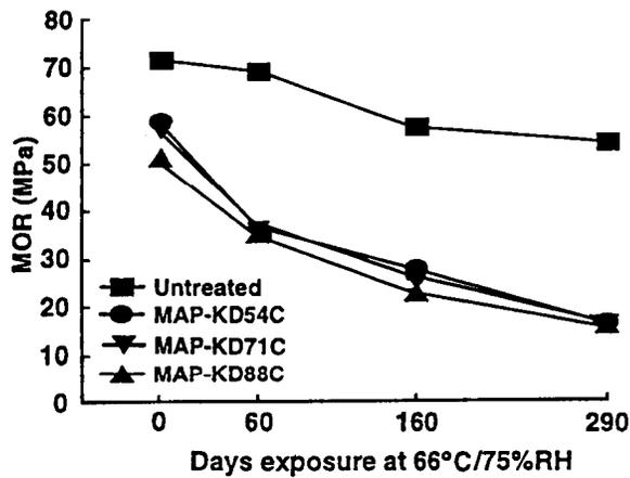
Figure 6. — Effects of redrying temperatures at 54°, 71°, or 88°C on bending strength of 12-mm-thick FR-treated plywood subsequently exposed to extended exposure at 66°C (22).
