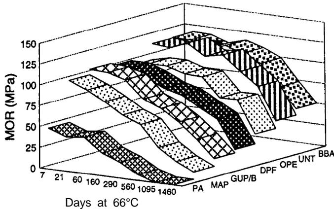
Figure 1. — Predicted change in bending strength over steady-state exposure of up to 4 years at 66°C for untreated (UNT) wood and wood treated with phosphoric acid (PA), monoammonium phosphate (MAP), guanylurea phosphate/boric acid (GUP/B), dicyandiamide-phosphoric acid-formaldehyde (DPF), organophosphonate ester (OPE), or borax/boric acid (BBA).
