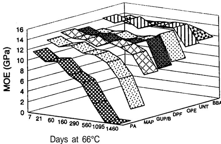
Figure 2. — Predicted change in modulus of elasticity (MOE) over steady-state exposure of up to 4 years at 66°C for untreated and treated wood.
