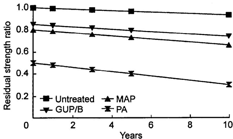
Figure 8. — Predicted change in residual strength ratio, defined as ratio of strength of treated to untreated wood, over a simulated 10-year exposure (25) in north central United States using kinetics-based models (8).
