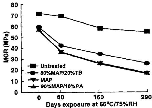
Figure 5. — Effects of FR treatment mixtures on bending strength of 12-mm-thick plywood subsequently exposed to extended exposure at 66°C (22).
