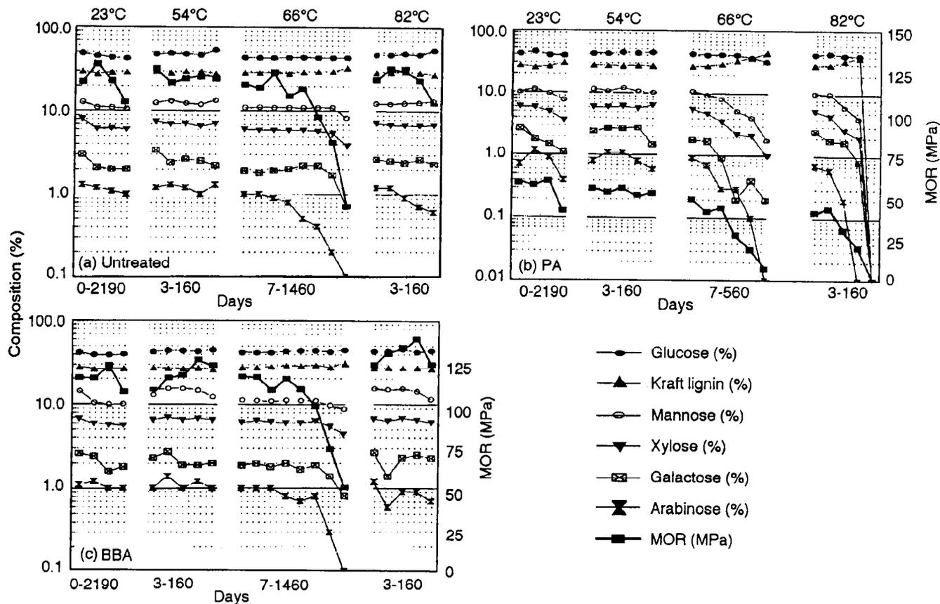
Figure 4.— Relationship between loss in bending strength (MOR) and changes in lignin content and content of individual carbohydrate components of hemicellulose and cellulose for untreated and treated wood (26).
