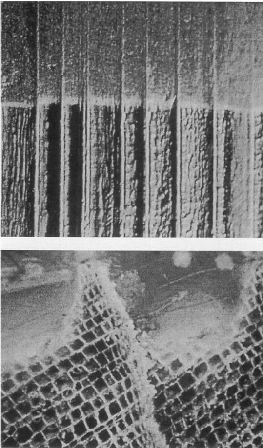
FIG. 9. Erosion of western redcedar. Top: weathered surface of wood; bottom: side view of a weathered surface showing differential erosion of earlywood and latewood.
