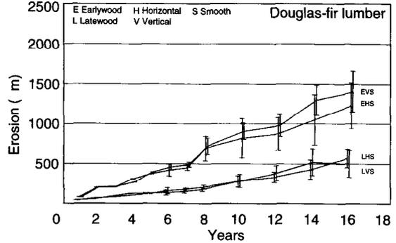
FIG. 6. Erosion of vertical-grained Douglas-fir lumber as a function of years of exposure (average of measurements on three replicate specimens).
