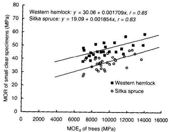
FIG. 9. Relationship of MOE<sub>d</sub> of trees to MOR of small, clear specimens.
