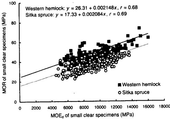
FIG. 6. Relationship of MOE<sub>d</sub> to MOR for small, clear specimens.
