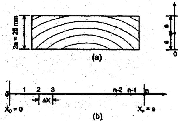
Figure 1. Test specimen and discretization of space co-ordinate. (a) Specimen with thickness in radial direction; (b) discretization of space coordinate with mesh width.
