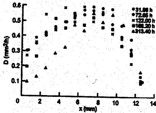
Figure 5. Variations of diffusion coefficient with space at various time points.
