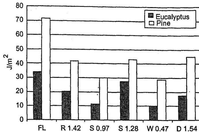
Fig. 3. Total energy absorption (TEA) values for handsheets from bleached eucalyptus and pine kraft pulps with 25% calcium carbonate fillers: fiber loaded, rhombohedral (1.42  $\mu\text{m}$  diam.), scalenohedral (0.97 and 1.28  $\mu\text{m}$ ), and wet ground (0.47  $\mu\text{m}$ ) and dry ground (1.54  $\mu\text{m}$ ).
