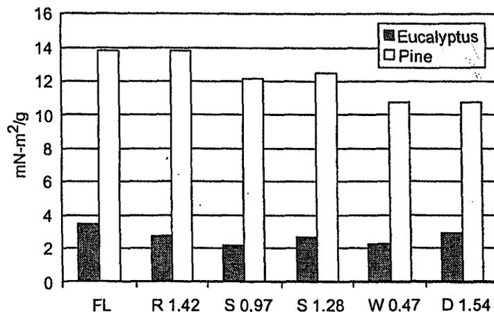
Fig. 4. Tear index values, for handsheets from bleached eucalyptus and pine kraft pulps with 25% calcium carbonate fillers: fiber loaded, rhonibohedral (1.42  $\mu\text{m}$  diam.), scalenohedral (0.97 and 1.28  $\mu\text{m}$ ), and wet ground (0.47  $\mu\text{m}$ ) and dry ground (1.54  $\mu\text{m}$ ).
