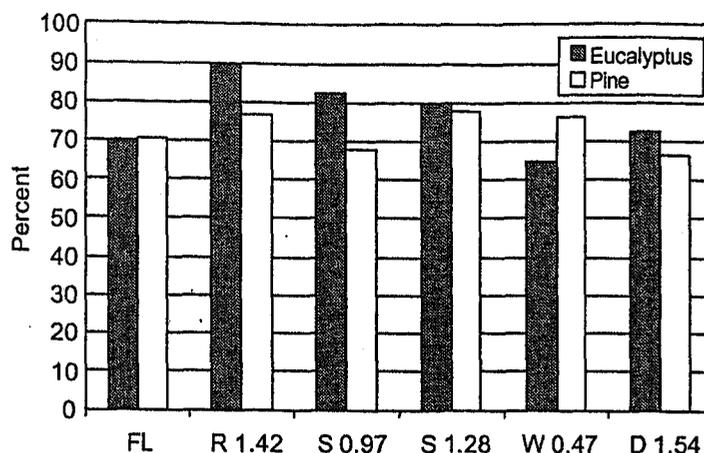
*Fig. 7. Diffuse scattering coefficient for handsheets from bleached eucalyptus and pine kraft pulps with 25% calcium carbonate fillers: fiber loaded, rhombohedral (1.42  $\mu\text{m}$  diam.), scalenohedral (0.97 and 1.28  $\mu\text{m}$ ), and wet ground (0.47  $\mu\text{m}$ ) and dry ground (1.54  $\mu\text{m}$ ).*
