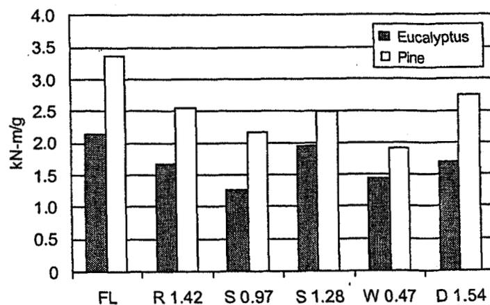
**Fig. 2. Tensile index values for handsheets from bleached eucalyptus and pine kraft pulps with 25% calcium carbonate fillers: fiber loaded, rhombohedral (1.42  $\mu\text{m}$  diam.), scalenohedral (0.97 and 1.28  $\mu\text{m}$ ), and wet ground (0.47  $\mu\text{m}$ ) and dry ground (1.54  $\mu\text{m}$ ).**
