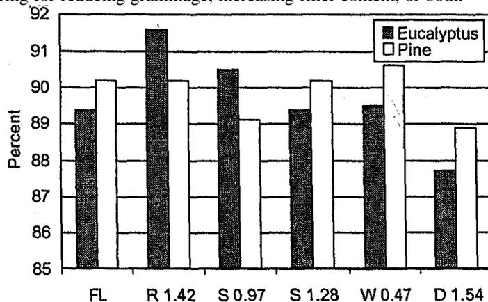
Fig. 6. Diffuse opacity for handsheets from bleached eucalyptus and pine kraft pulps with 25% calcium carbonate fillers: fiber loaded, rhombohedral (1.42  $\mu\text{m}$  diam.), scalenohedral (0.97 and 1.28  $\mu\text{m}$ ), and wet ground (0.47  $\mu\text{m}$ ) and dry ground (1.54  $\mu\text{m}$ ).
