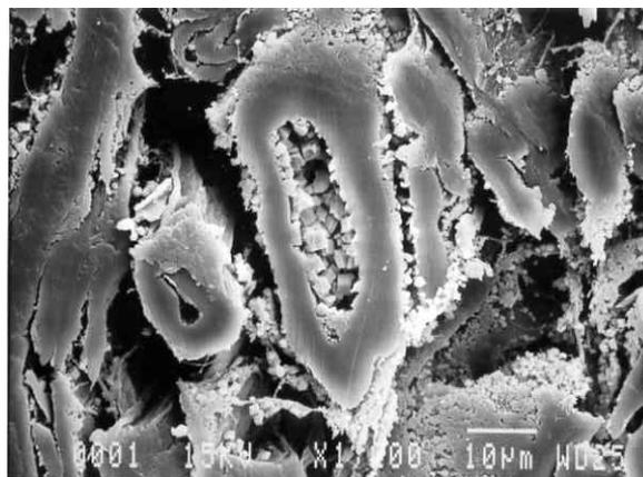
*Fig. 1. Scanning electron microscope (SEM) micrograph of handsheet cross section. This micrograph shows fiber-loaded precipitated calcium carbonate (FLPCC) deposited within, on the surface of, and outside the pulp fibers.*
