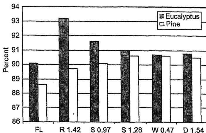
Fig. 5. Diffuse brightness values for handsheets from bleached eucalyptus and pine kraft pulps with 25% calcium carbonate fillers: fiber loaded, rhombohedral (1.42  $\mu\text{m}$  diam.), scalendhedral (0.97 and 1.28  $\mu\text{m}$ ), and wet ground (0.47  $\mu\text{m}$ ) and dry ground (1.54  $\mu\text{m}$ ).
