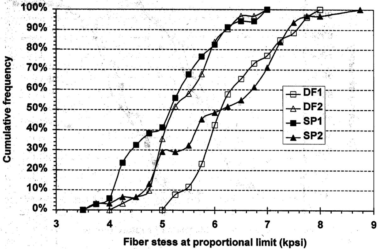
Figure 3. Cumulative frequency diagram for fiber stress of  $3\frac{1}{2} \times 4\frac{1}{2}$ -in (1) and  $3\frac{3}{4} \times 4\frac{3}{4}$ -in (2) southern pine (SP) and Douglas-fir (DF) crossarms.
