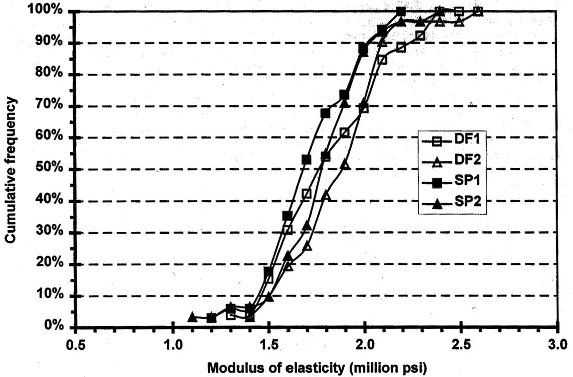
Figure 1. Cumulative frequency diagram for modulus of elasticity of 3 1/2 x 4 1/2-in (1) and 3 3/4 x 4 3/4-in (2) southern pine (SP) and Douglas-fir (DF) crossarms.
