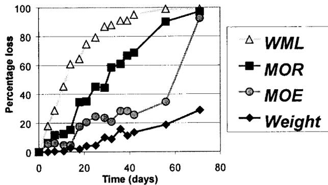
**Figure 6.**—Effect of decay by *G. trabeum* on weight loss and mechanical properties.
