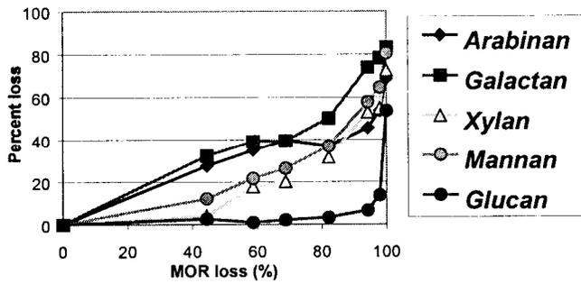
**Figure 5.**—Comparison of loss of carbohydrate components with loss in bending strength (MOR) caused by *G. trabeum*.
