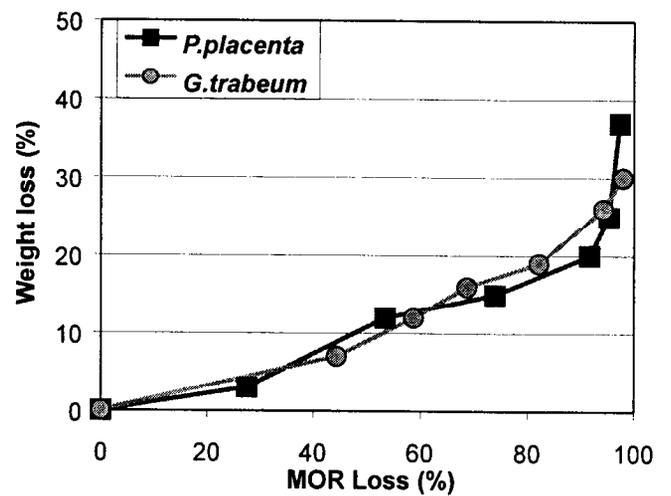
Figure 3.—Comparison of brown rot induced bending strength (MOR) and weight loss in southern pine.
