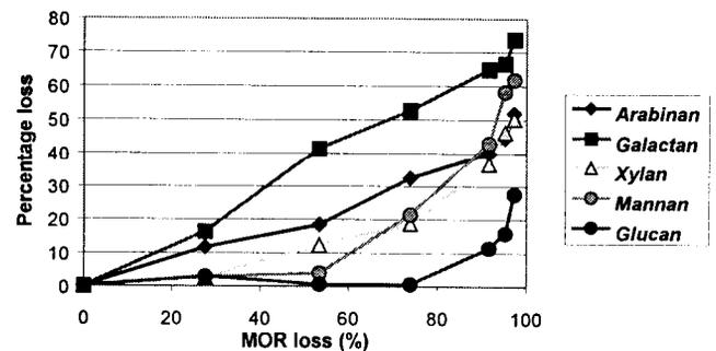
Figure 4.—Comparison of loss of carbohydrate components with loss in bending strength (MOR) caused by *P. placenta*.
