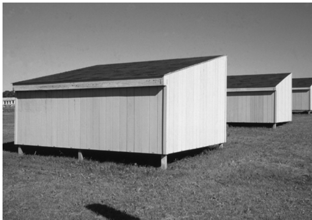
Figure 7. Field chambers for roof temperature studies in Wisconsin (Northern US) and Mississippi (Southern US).
