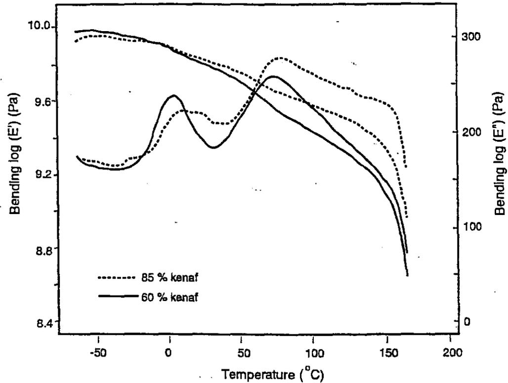
**Figure 2. Storage and loss modulus of a 85 % fiber filled composite compared to injection molded 60 % fiber filled composite.**
