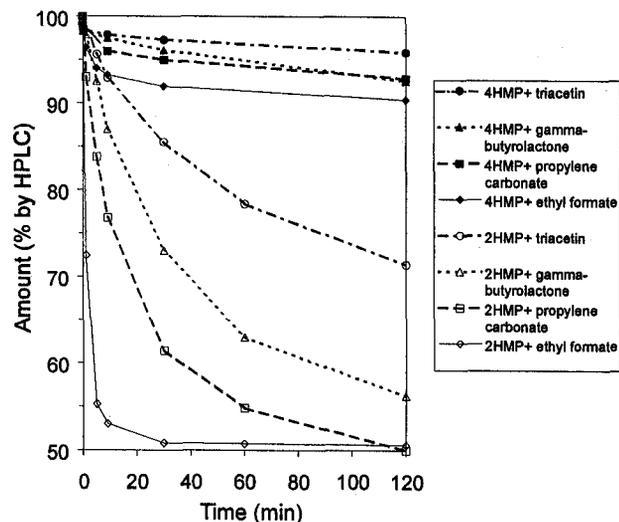
**Figure 5.** –Comparison of the rates of disappearance of 2-HMP and 4-HMP reacted with cure accelerators under the same reaction conditions.
