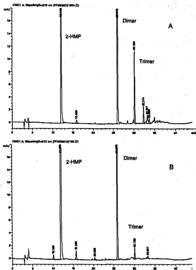
**Figure 3.**—HPLC chromatograms of (A) 2-HMP reacted at 20°C with a cure accelerator and (B) 2-HMP reacted at 60°C without a cure accelerator.
