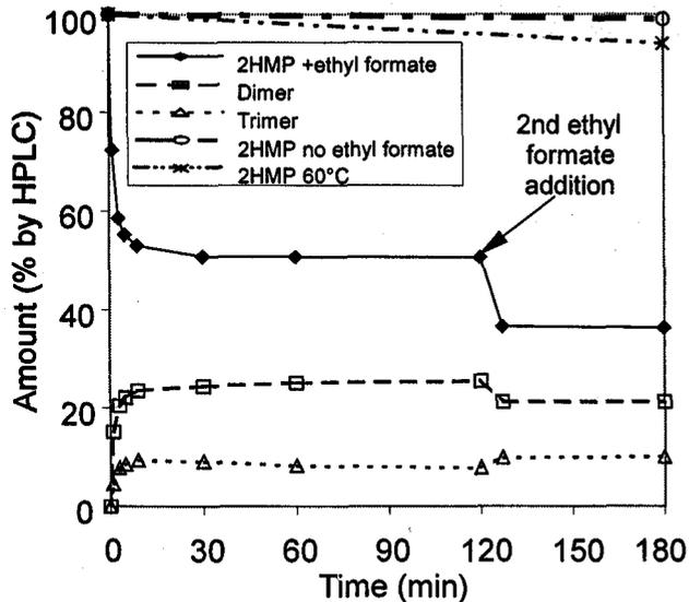
**Figure 1.**—The effect of ethyl formate on the condensation of 2-HMR
