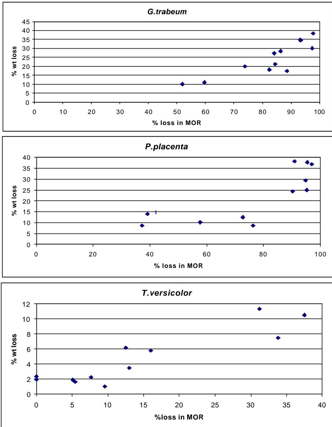
**Figure 4.** Relationship between weight loss and strength loss
