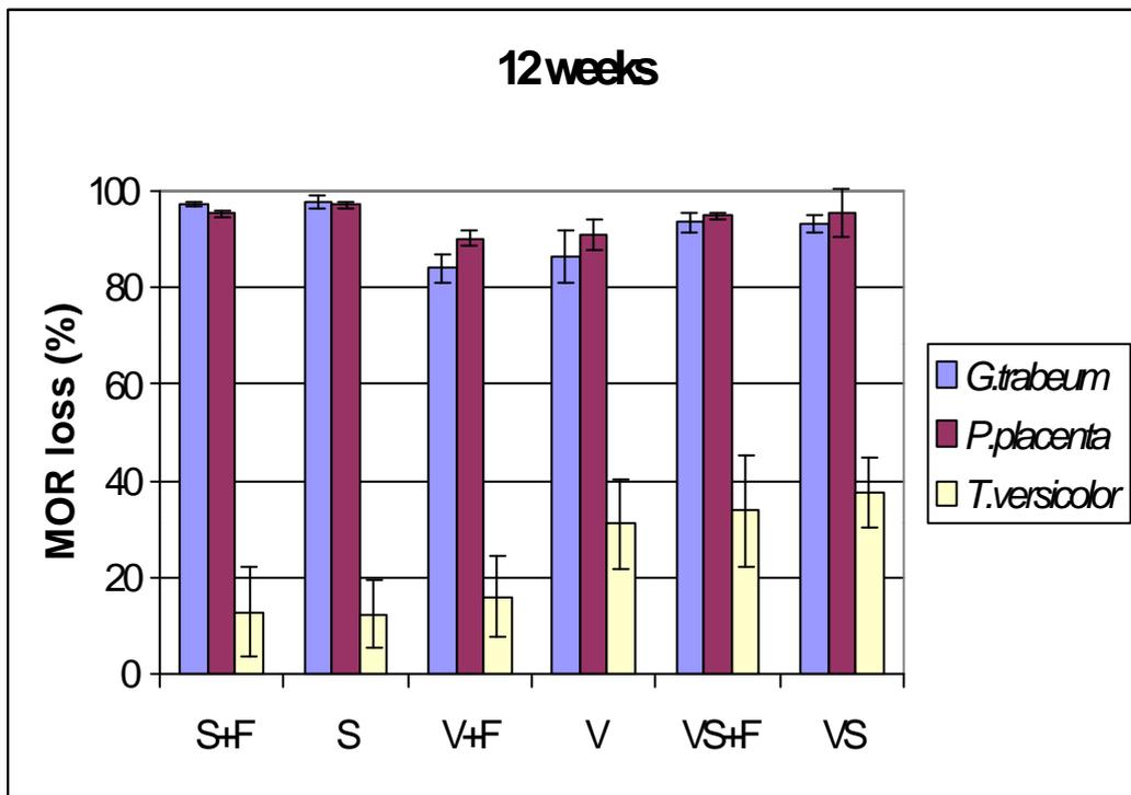
**Figure 3** Strength loss of samples after exposure to decay fungi for 6 and 12 weeks. (error bars show 95% confidence intervals) (S + F = soil and feeder, S = Soil, V +F = vermiculite and feeder, V = vermiculite VS + F = vermiculite/soil and feeder, VS = vermiculite/soil)
