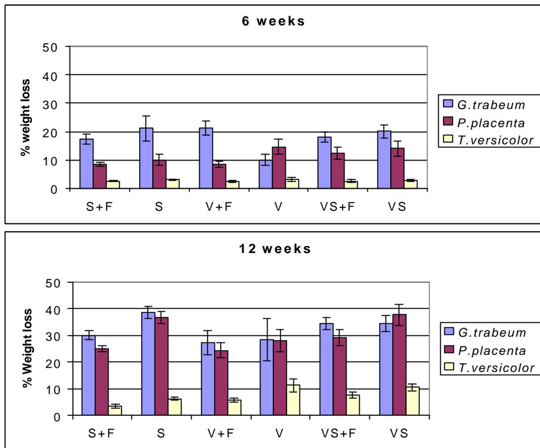
**Figure 2** Mean weight loss of samples after exposure to decay fungi for 6 and 12 weeks. (error bars show 95% confidence intervals) (S + F = soil and feeder, S = Soil (no feeder), V +F = vermiculite and feeder, V = vermiculite (no feeder)VS + F = vermiculite/soil and feeder, VS = vermiculite/soil (no feeder))
