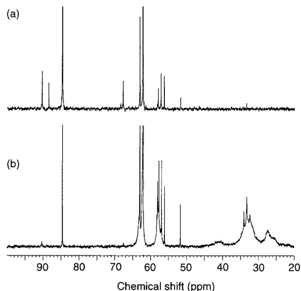
**Figure 6** Carbon-13 NMR spectrograms of HMR, using <sup>13</sup>C-enriched formaldehyde, obtained from reaction times between: (a) 4 and 12 min and (b) 7.3 and 9.3 h.
