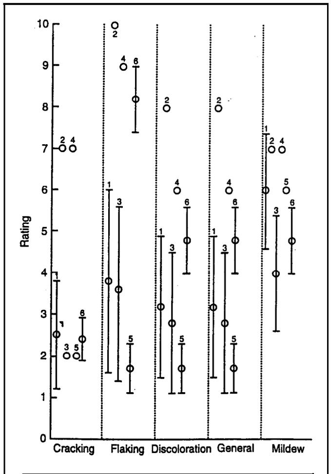
Figure 7—Comparison of mean ratings and standard deviations for Finishes 1 through 6 in each of the five evaluation categories after 11 years exterior exposure near Madison, WI (Finishes 1, 3, and 5 are alkyd based; Finishes 2, 4, and 6 are latex based).
