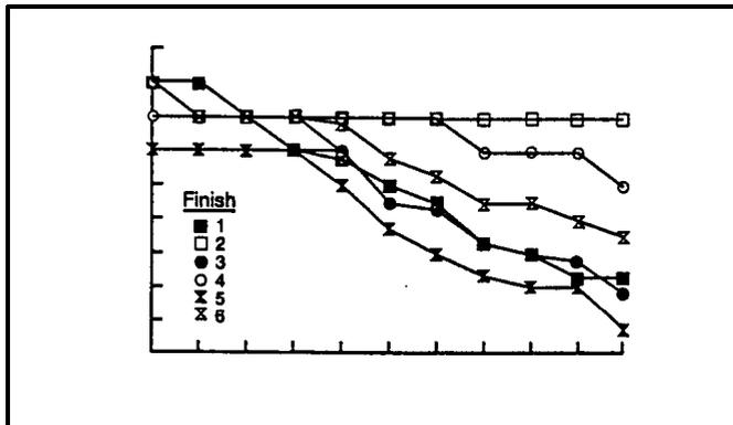
Figure 4—Average discoloration rating for the finishes during 11 years (panels finished in 1985) of exterior exposure near Madison, WI. 10 = no degradation; 5 = point at which refinishing should be done; 1 = complete failure of finish (Finishes 1, 3, and 5 are alkyd based; Finishes 2, 4, and 6 are latex based).
