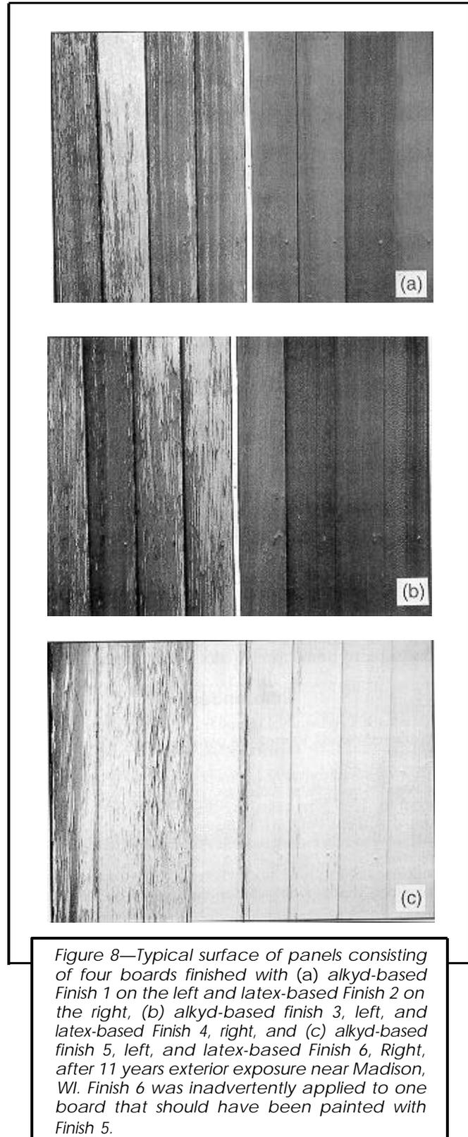
Figure 8—Typical surface of panels consisting of four boards finished with (a) alkyd-based Finish 1 on the left and latex-based Finish 2 on the right, (b) alkyd-based finish 3, left, and latex-based Finish 4, right, and (c) alkyd-based finish 5, left, and latex-based Finish 6, Right, after 11 years exterior exposure near Madison, WI. Finish 6 was inadvertently applied to one board that should have been painted with Finish 5.
