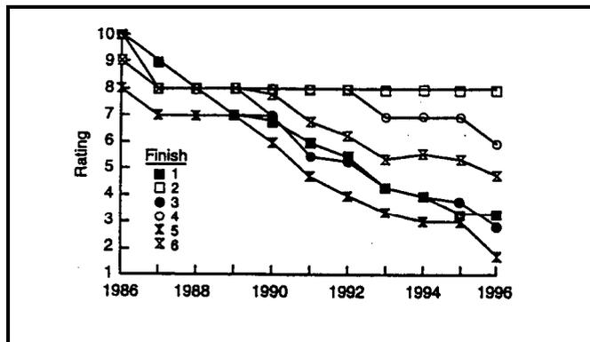
Figure 5—Average general rating for the finishes during 11 years (panels finished in 1985) of exterior exposure near Madison, WI. 10 = no degradation; 5 = point at which refinishing should be done; 1 = complete failure of finish (Finishes 1, 3, and 5 are alkyd based; Finishes 2, 4, and 6 are latex based).
