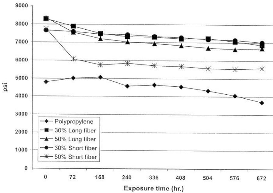
**Figure 1.** ~ Flexural strength versus exposure for four types of agroplastics and polypropylene.
