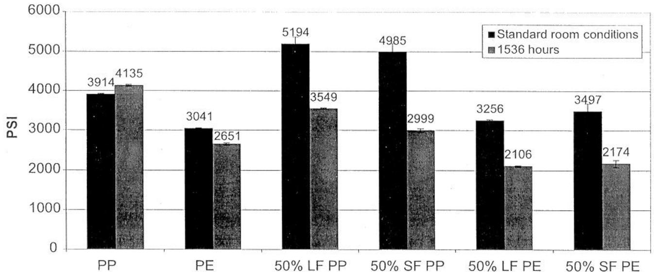
**Figure 7.** ~ Effects of water absorption on tensile strength. PP = polypropylene; PE = polyethylene; LF = long fiber; and SF = short fiber.
