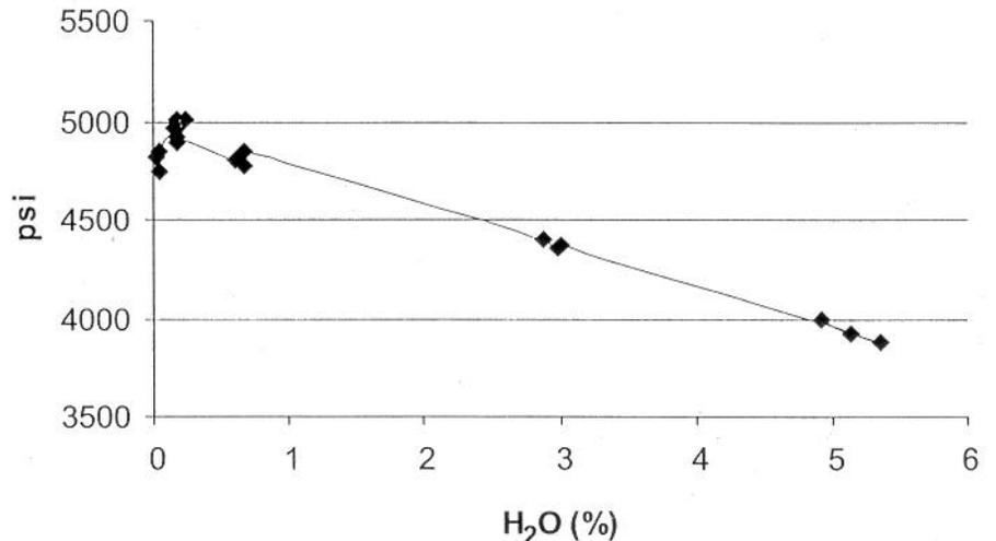
**Figure 8.** ~ Correlation of water absorption with tensile strength.
