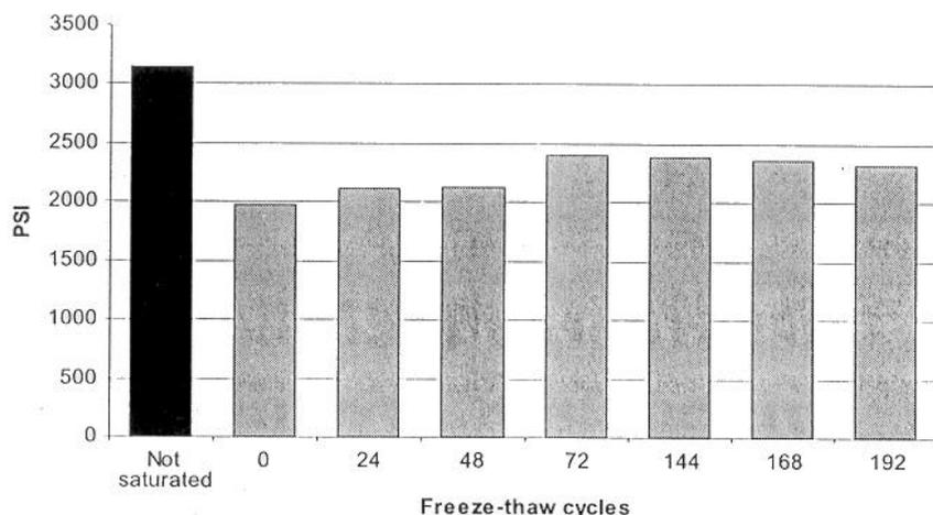
**Figure 9.** ~ Effect of freeze-thaw cycles on tensile strength of 50 percent polyethylene long-fiber agroplastics.
