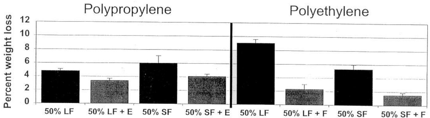
**Figure 5.** ~ Percent loss of agrocomposites after 3 months of exposure to fungal decay. Two treatments were used to prevent fungal attack. LF = long fiber; SF = short fiber.
