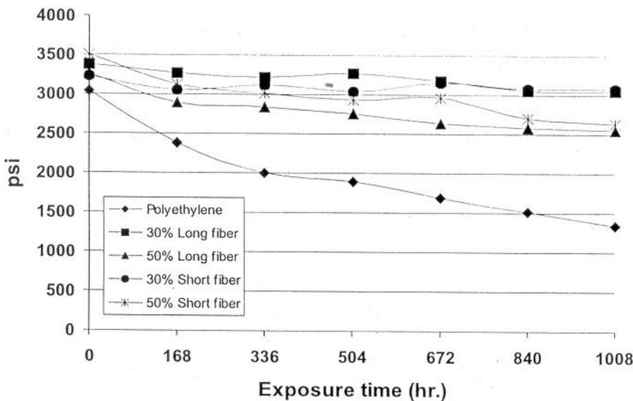
**Figure 2.** ~ Tensile strength versus exposure for agrocomposites and polyethylene.
