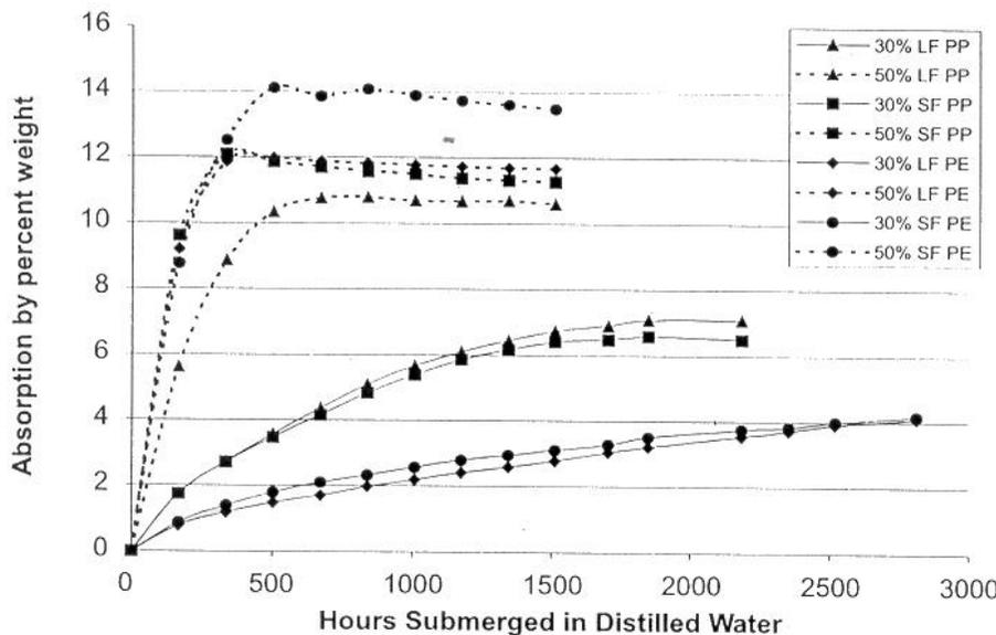
**Figure 6.** ~ Rates of water absorption for different types of agroplastics. Polypropylene (PP) and polyethylene (PE) had zero water absorption. LF = long fiber; SF = short fiber.
