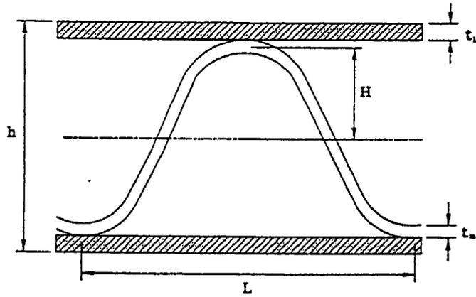
Figure 2 - Corrugated Board Key Dimensions
