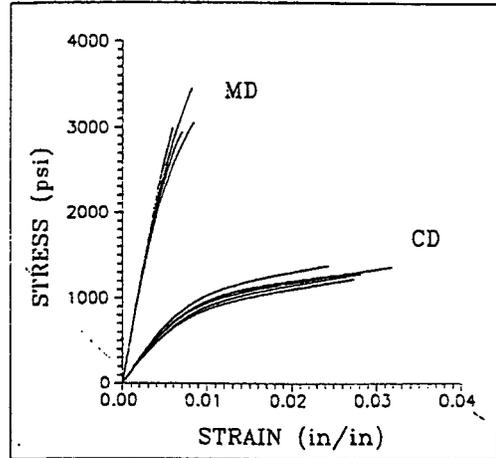
Figure 3 - Stress-Strain Curves (Tension, Liner)
