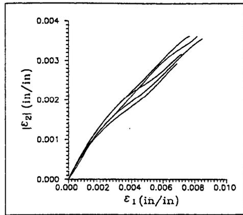
Figure 4 - Poisson's Ratio Test Data (MD Extension, Liner)
