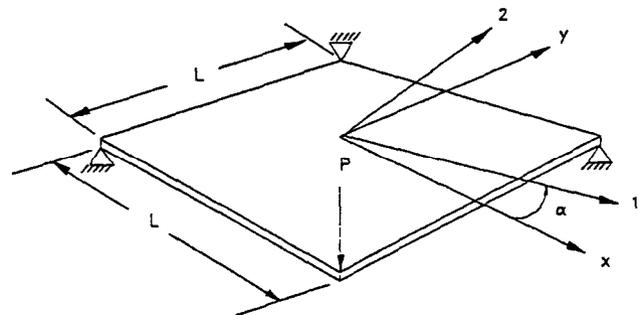
Figure 10 - Schematic of Pure Twisting Test Loading Geometry
