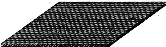
Figure 12 - Twisting Test Finite Element Mesh
