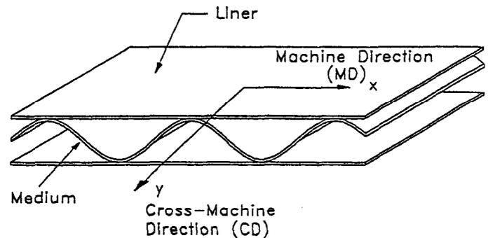
Figure 1- Corrugated Board Structure
