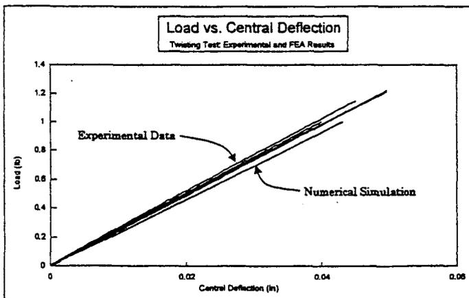
Figure 13 - Correlation of FEA Predictions with Experimental Data for the Anticlastic Plate Twisting Test Geometry
