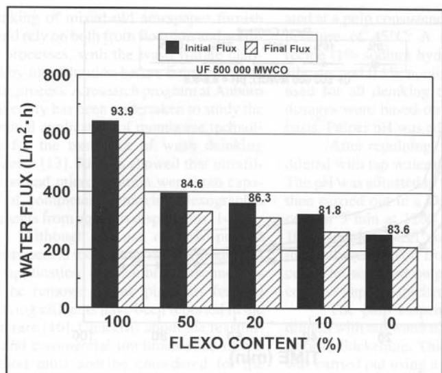
Fig. 3 Pure water permeation rate before experimentation and after cleaning the ultrafiltration membrane. Values reported on the top of the bars are the cleaning efficiency  $E_C$  of the membrane after processing feed effluents.
