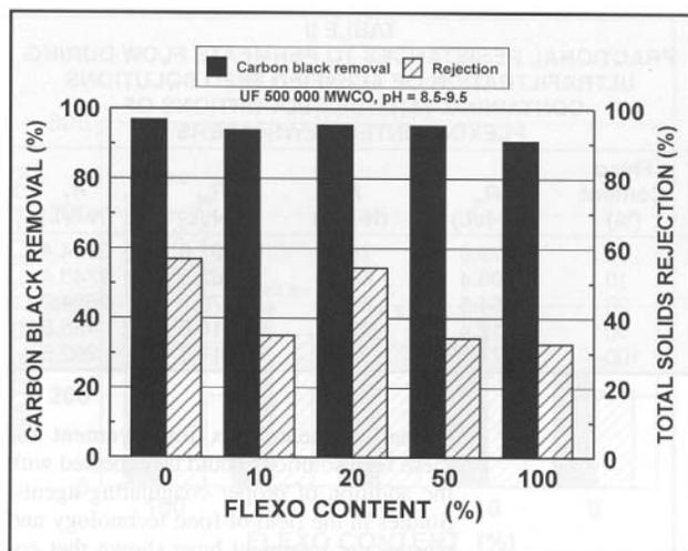
Fig. 5. Carbon black removal efficiency and rejection of total solids by ultrafiltration for alkaline feed solutions containing various proportions of flexo-printed newspapers.
