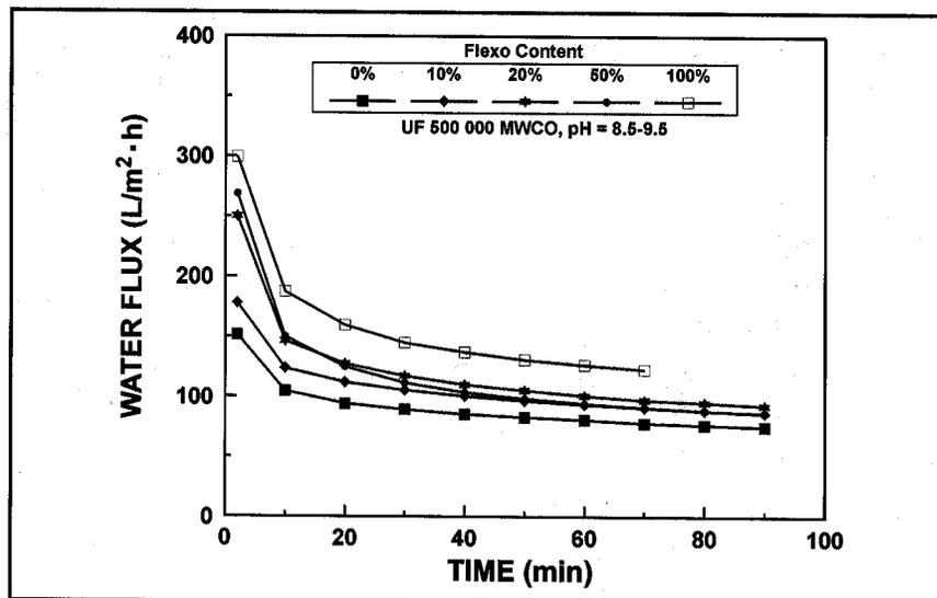
Fig. 2. Permeate flux decline for feed solutions containing various proportions of flexo-printed newspapers.
