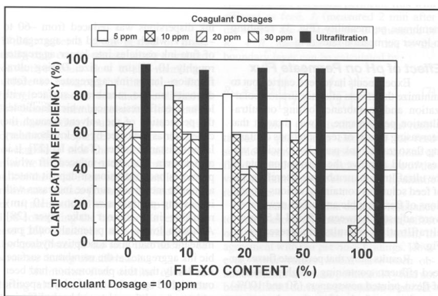
Fig. 7. Clarification efficiency for ultrafiltration and standard jar tests for feed solutions containing various proportions of flexo-printed newspapers.
