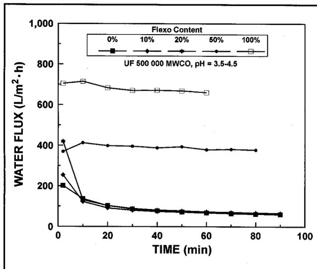
Fig. 4. Permeate flux for feed solutions containing various proportions of flexo-printed newspapers. Feed effluents were acidified between pH 3.5 and 4.5 before ultrafiltration.
